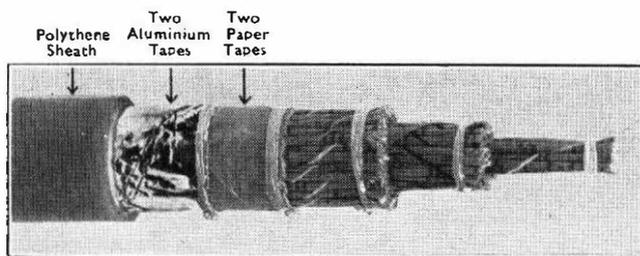
FIG. 19.—EXPERIMENTAL 54-PAIR POLYTHENE-SHEATHED CABLE WITH ALUMINIUM CONDUCTORS.
