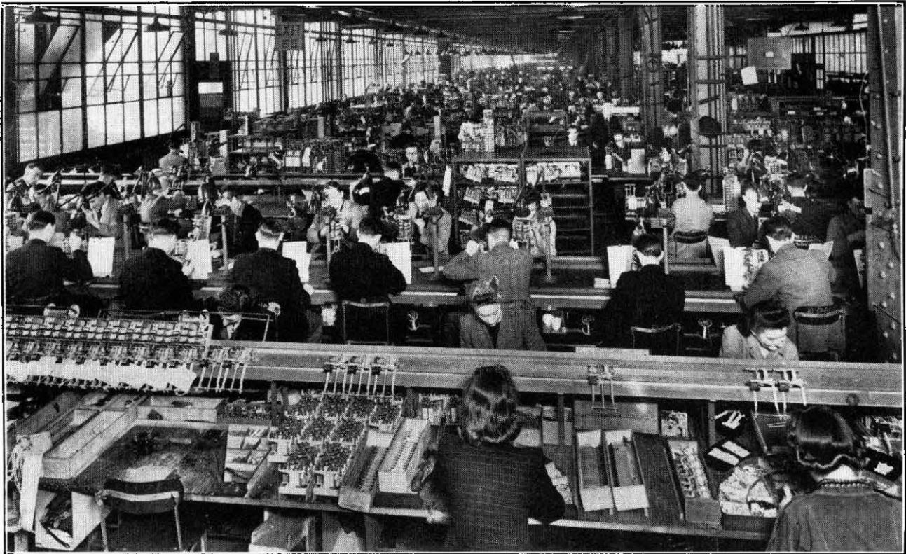
MAIN ASSEMBLY AND WIRING OF 2,000-TYPE SELECTORS.
