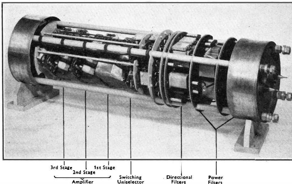
FIG. 11.—EARLY SUBMERGED TELEPHONE REPEATER.
