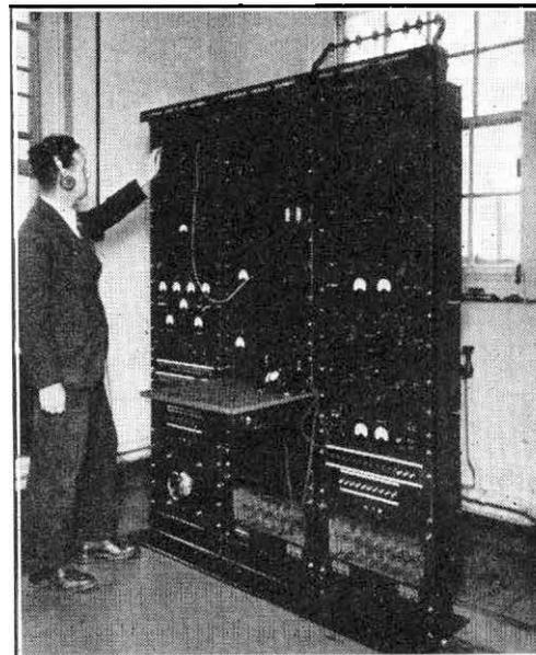
FIG. 5.—SHORT-WAVE TELEPHONY RECEIVER AT BALDOCK RADIO STATION.
