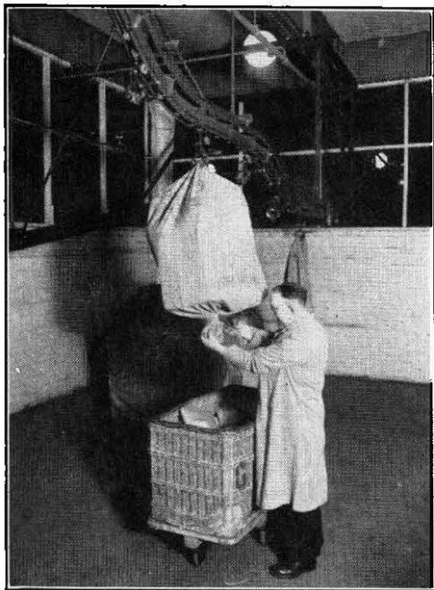
FIG. 4.—BAG OPENING FROM A CHAIN CONVEYOR.
