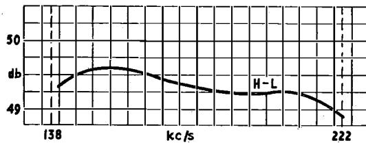
FIG. 16.—TYPICAL REPEATER CONVERSION GAIN/FREQUENCY RESPONSE.
