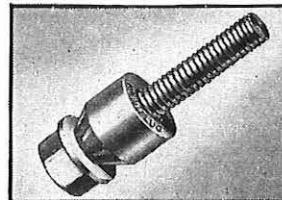
Use Rawlplug BOLT ANCHORS for bolting down in extremely wet or corrosive situations. Caulking completely seals the anchorage. Use also for anchoring Diesel Generators, Power Hammers, etc.
