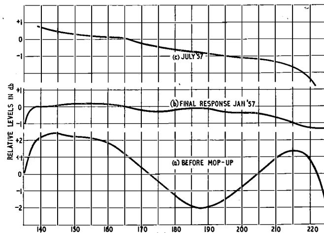
FIG. 18.—TYPICAL LINE ATTENUATION/FREQUENCY RESPONSES MEASURED BETWEEN SUB-GROUP COMMON POINTS.
