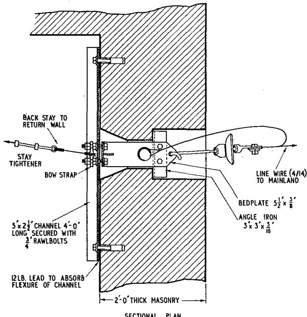
FIG. 3.—STEELWORK AND INSULATOR FIXING AT THE PARAPET WALL ON THE FORT.
