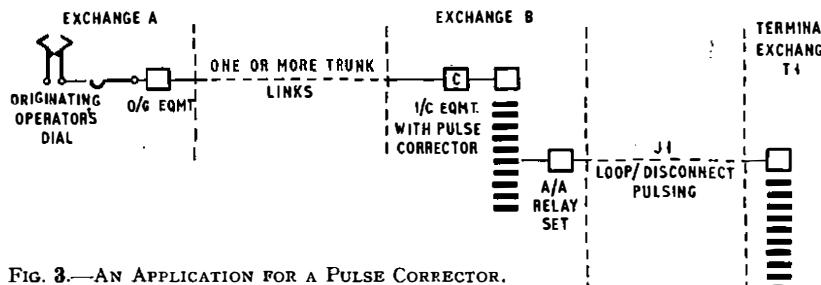
FIG. 3.—AN APPLICATION FOR A PULSE CORRECTOR.
