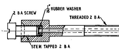
FIG. 5.—HOLLOW PRESSURE-TESTING BOLT.
