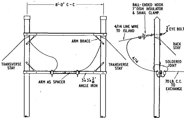
FIG. 4.—32-FT MEDIUM TWIN POLE ASSEMBLY ON MAINLAND.
