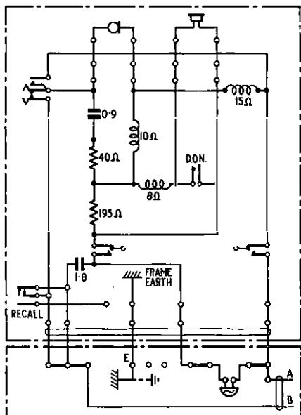
FIG. 5.—CIRCUIT OF THE 1,000-OHM FLAMEPROOF TABLE TELEPHONE.
