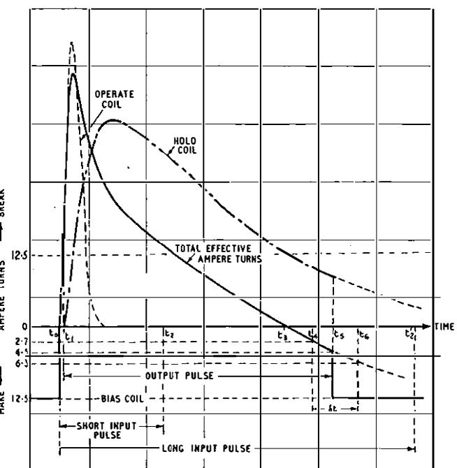
FIG. 8.—VARIATIONS OF AMPERE-TURNS DURING ONE CYCLE.
