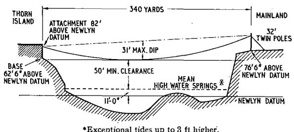
FIG. 2.—SPAN PROFILE.
