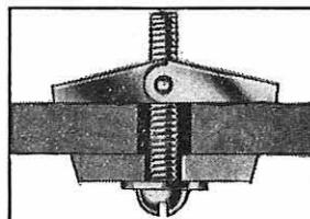
For ceilings of lath and plaster, plasterboard, etc., use Rawlplug SPRING TOGGLS. The inserted Toggle springs open behind the material, spreading the load over a wide area.
