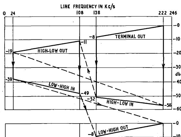
FIG. 8.—LINE TEST LEVEL DIAGRAM CALCULATED FOR SIX-MILE SECTIONS OF 20-LB. P.C.Q.T. CABLE.
