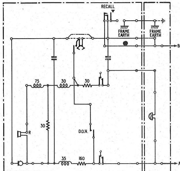
FIG. 4.—CIRCUIT OF THE 600-OHM FLAMEPROOF TABLE TELEPHONE.
