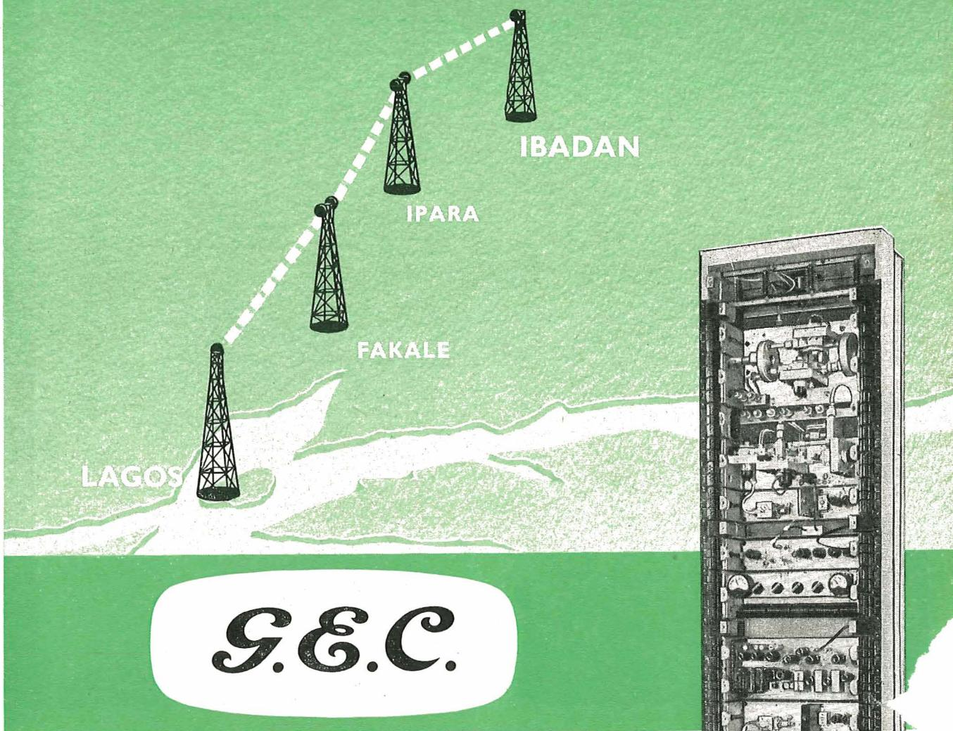
Continuing its progressive policy of telephone communications development, the Government of Nigeria has ordered a G.E.C. microwave radio-telephone system to provide service between Lagos and Ibadan. G.E.C. 240-circuit 2000 Mc/s radio-relay equipment, together with G.E.C. carrier-telephone equipment, will provide 480 speech circuits and a spare radio channel arranged to give automatic standby facilities. A complete radio transmitter and receiver is mounted on one 7' 6" rackside.
