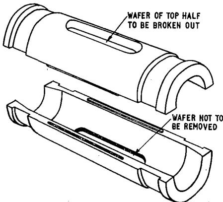
FIG. 3.—WATER-BARRIER COUPLING.
