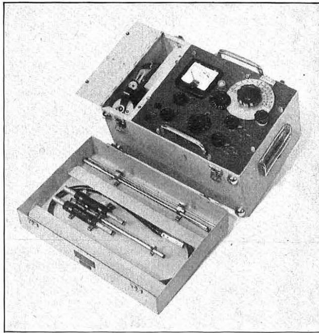
FIG. 2.—RECEIVER, RADIO, NO. 12 (30 TO 100 Mc/s).
