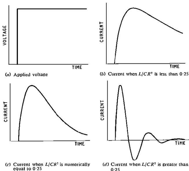
FIG. 1—STEP RESPONSE OF R, L, C CIRCUIT
