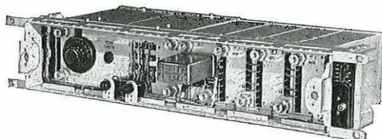
The associated frequency generating apparatus is controlled by a master oscillator (shown left) of high stability. Duplicate equipment is supplied and this together with automatic changeover provides a service of extreme reliability. Frequency checking, monitoring and alarm facilities are incorporated in the equipment and the whole carrier supply apparatus can be readily extended to meet all carrier supply requirements from 12 channels upwards.
