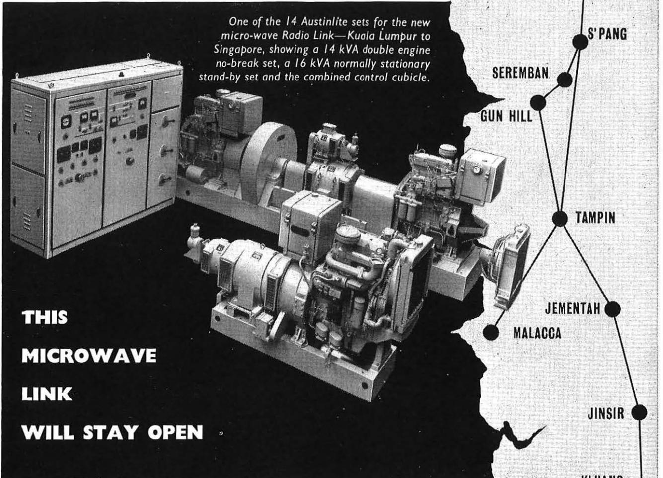
One of the 14 Austinlite sets for the new micro-wave Radio Link—Kuala Lumpur to Singapore, showing a 14 kVA double engine no-break set, a 16 kVA normally stationary stand-by set and the combined control cubicle.
