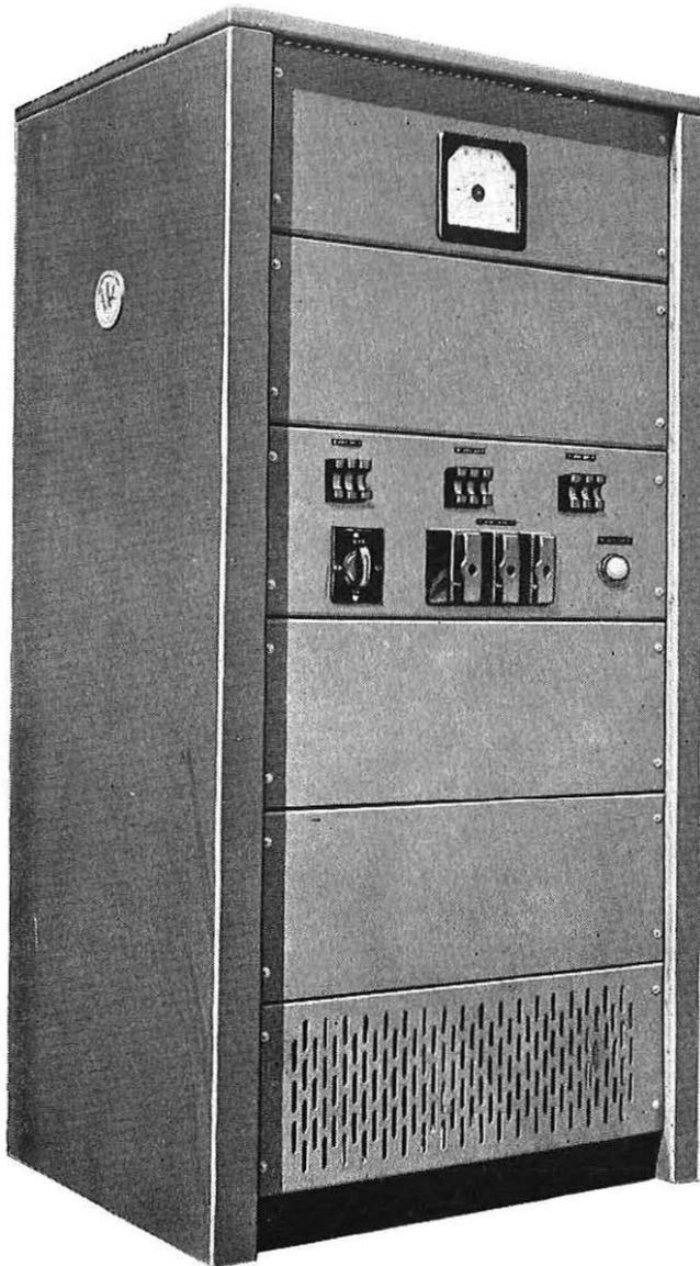
A Westinghouse transducer controlled rectifier set forms the basis of the power supply to the register translator in the new subscriber trunk dialling system. Equipments of this type are designed to stabilise the d.c. output voltage to less than  $\pm 1\%$  over a load range of 10% full load to full load despite simultaneous mains input voltage variations of  $\pm 6\%$  and frequency changes of  $+1\%$  to  $-2\%$ .
