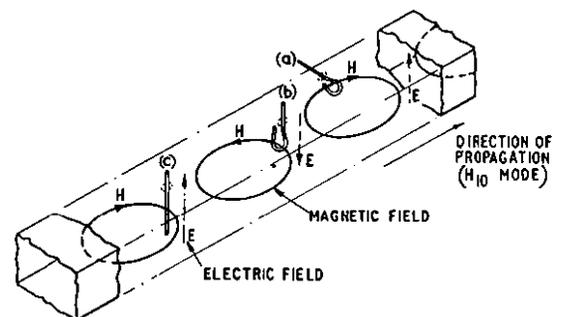
(a) Loop in the narrow side of guide, coupling with the magnetic field.
