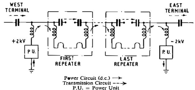
FIG. 2.—SUBMARINE-CABLE POWER-FEEDING ARRANGEMENTS (TAT-1)
