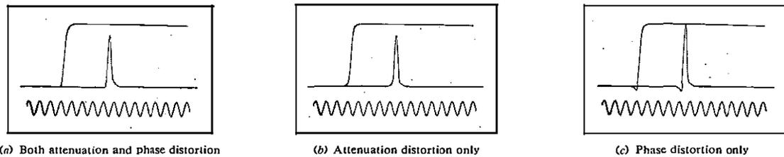
FIG. 12—WAVEFORM RESPONSES OF ATTENUATION AND PHASE DISTORTIONS
