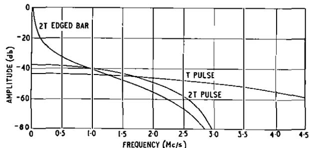
The ordinates are the peak-to-peak amplitudes of the spectral components in decibels relative to the peak-to-peak amplitude of the waveform.
