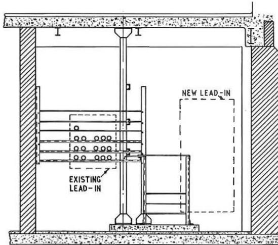
EXISTING CABLES SUPPORTED ON ADDITIONAL BEARERS IN NEW CABLE CHAMBER
