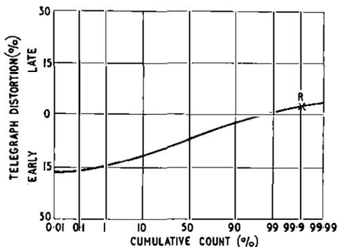
FIG. 1.—DISTORTION MEASURED ON A TYPICAL CIRCUIT
