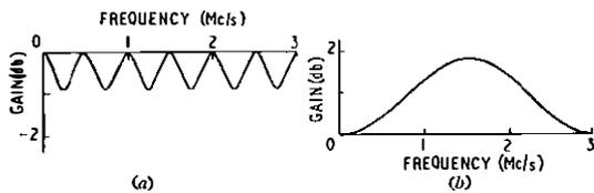
FIG. 8—GAIN/FREQUENCY RESPONSES OF ECHO DISTORTIONS
