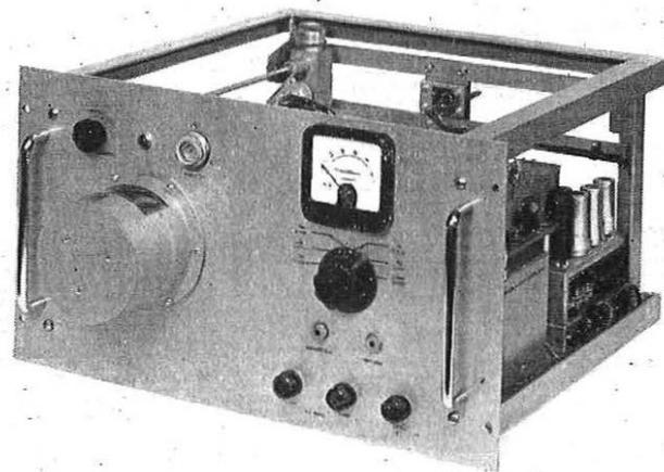
FIG. 3—CAVITY-CONTROLLED MICROWAVE CARRIER SOURCE
