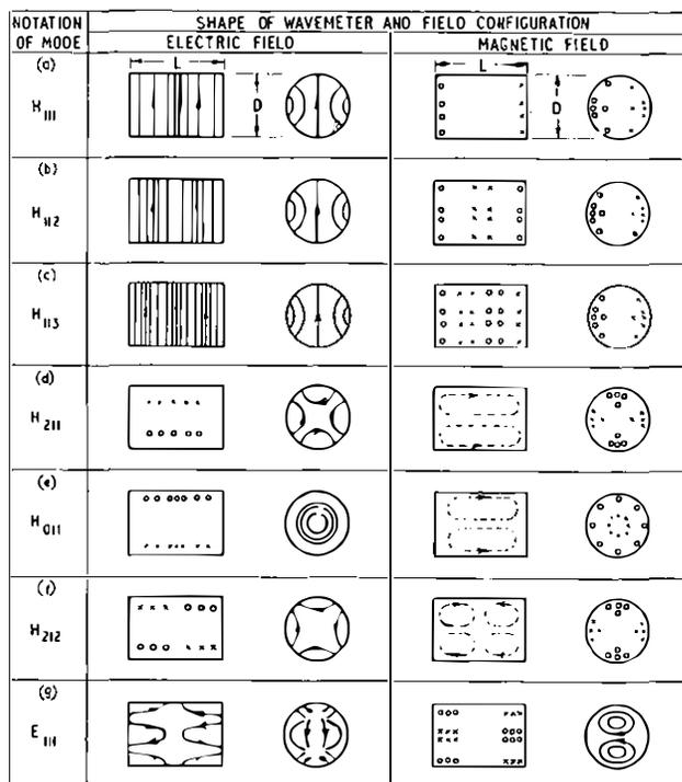
Electric and magnetic fields are in time quadrature if the effects of losses be neglected
