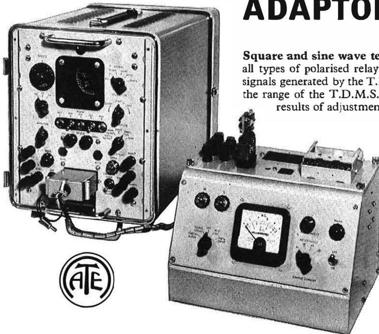
**Square and sine wave testing.** This adaptor is designed to check all types of polarised relays for bias and transit time, using the test signals generated by the T.D.M.S.5 series at signalling speeds within the range of the T.D.M.S., a visual indication of the condition and results of adjustment being indicated on the T.D.M.S.5.
