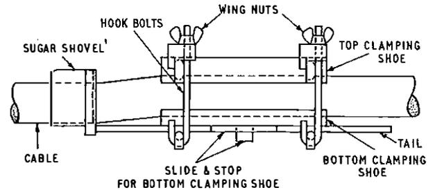
FIG. 6—EXPERIMENTAL SELF-CLAMPING ANTI-CREEPAGE DEVICE
