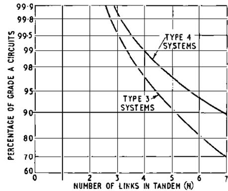
Grade A Circuits—those of performance better than that signified by a degree of inherent distortion of 30 per cent ( $P = 0.0001$ )
