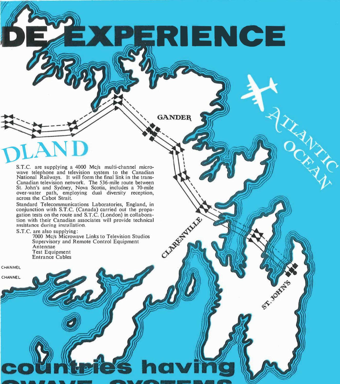
S.T.C. are supplying a 4000 Mc/s multi-channel microwave telephone and television system to the Canadian National Railways. It will form the final link in the trans-Canadian television network. The 536-mile route between St. John's and Sydney, Nova Scotia, includes a 70-mile over-water path, employing dual diversity reception, across the Cabot Strait.
