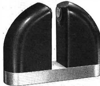
Another example, illustrated above, shows a fully protected 'horn' shaped magnet which gives a magnetic field in the gap of 5500 oersteds and weighs only 14 lb. A particular feature of this magnet is that it is specially designed to give an accurate and stable performance under the worst possible condition of usage. It can be brought into contact with iron and steel and other magnets and still remain within the manufacturer's specification and retain its magnetic calibration.
