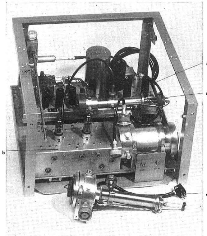
(a) 50 Mc/s quartz crystal in oven (sub unit)
