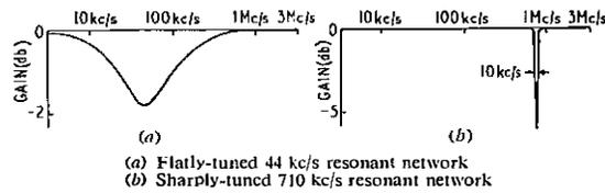
FIG. 6—GAIN/FREQUENCY RESPONSES OF RESONANT NETWORKS
