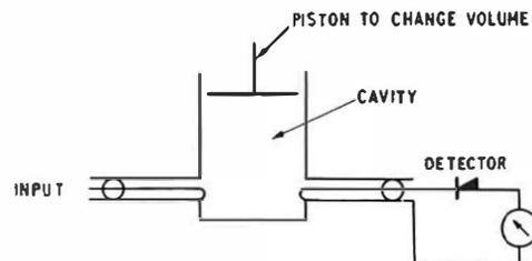
FIG. 2—PRINCIPLE OF CAVITY FREQUENCY-METER
