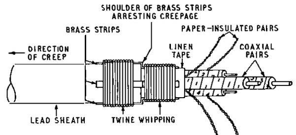
(a) Anti-creepage device for coaxial cables having few paper-insulated pairs
