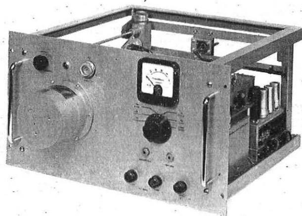
FIG. 3—CAVITY-CONTROLLED MICROWAVE CARRIER SOURCE
