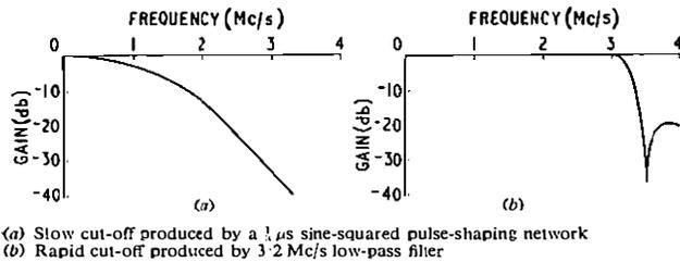
FIG. 10—GAIN/FREQUENCY RESPONSES OF BAND-WIDTH-RESTRICTING NETWORKS
