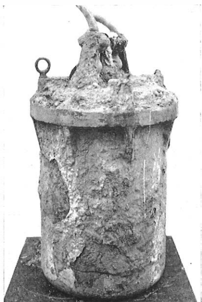
FIG. 2--TYPICAL CAST-IRON LOADING POT AS RECEIVED FOR REPAIR
