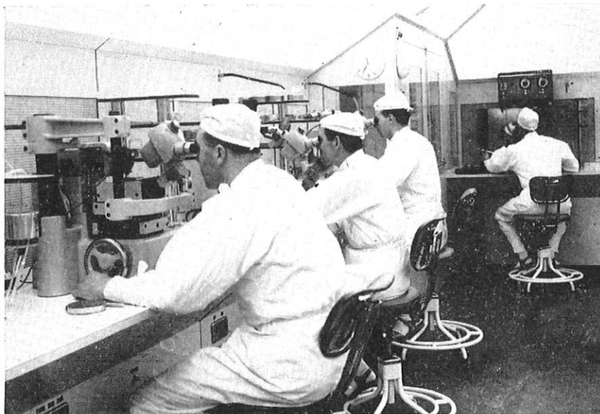
FIG. 5—TWO-PROBE TESTING, DICING, HEADING AND WIRE-BONDING POSITIONS
