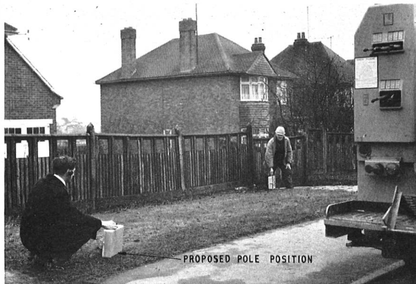
FIG. 3—LOCATOR No. 1A BEING USED TO CHECK A PROPOSED POLE POSITION
