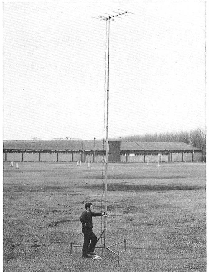
FIG. 6—Operator erecting the pneumatic mast for use remote from the vehicle
