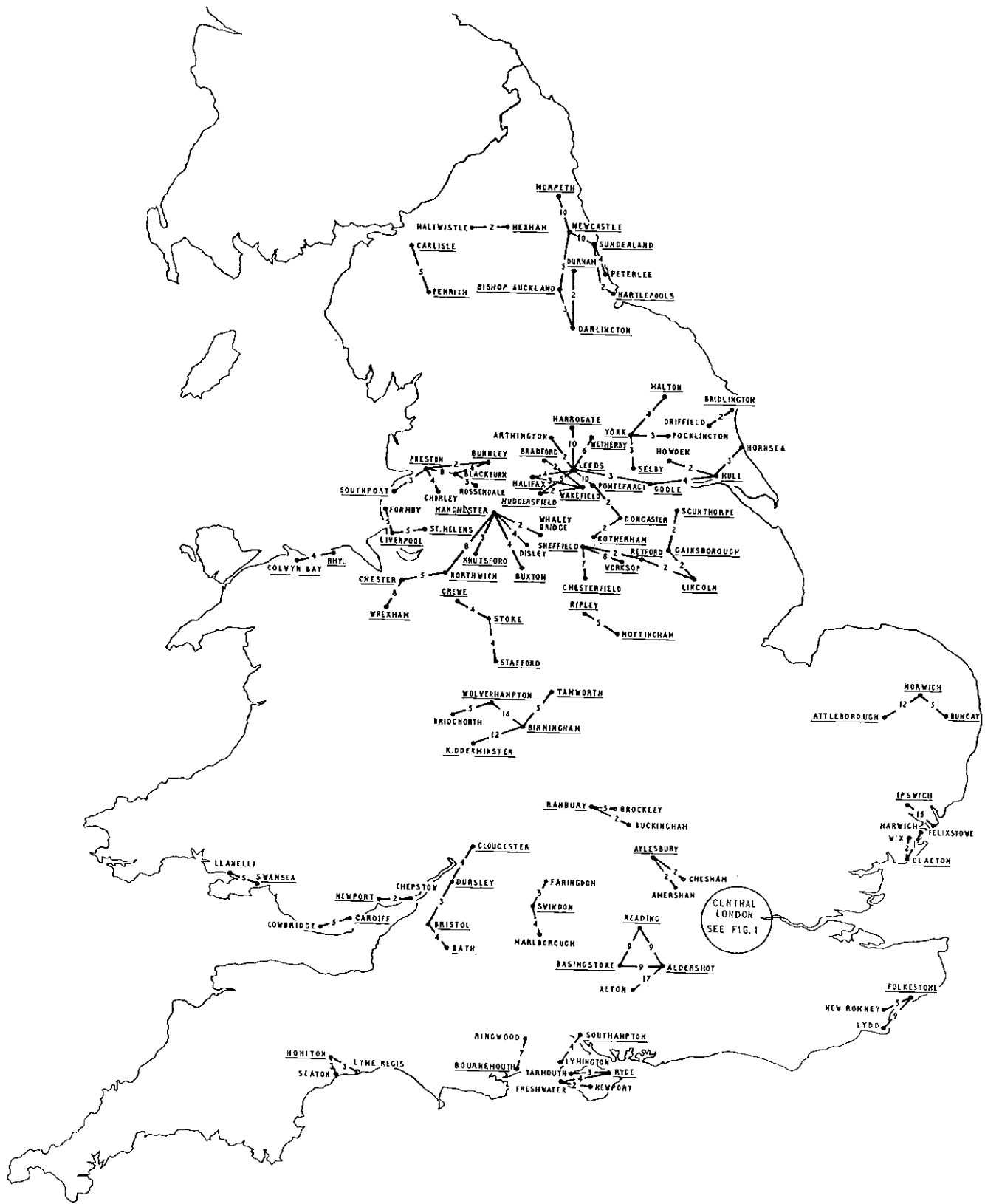
Fig. 2—24-circuit p.c.m. systems to be provided in England and Wales
