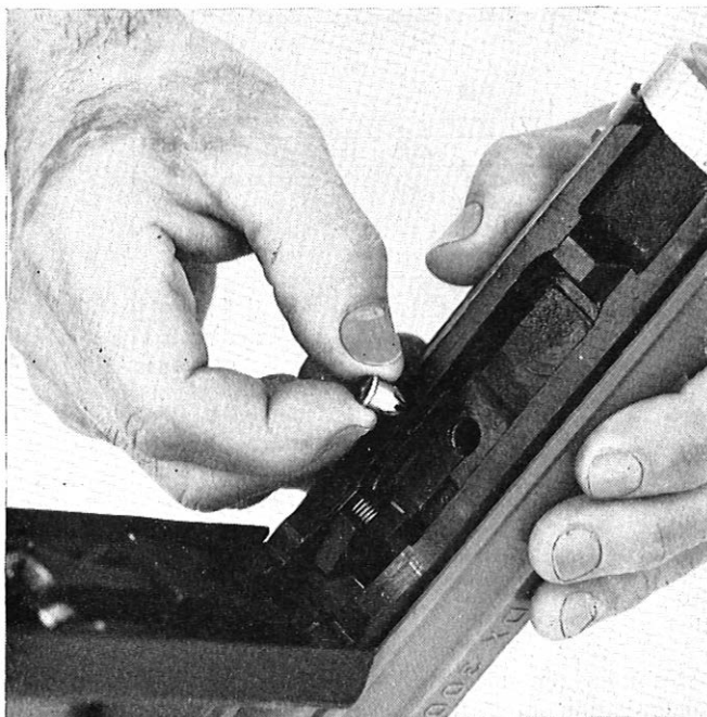
FIG. 3—Inserting cartridge in new-type tool
