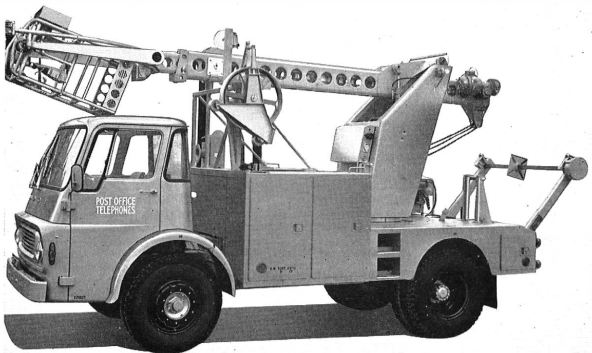
FIG. 1—Aerial-cable erection unit
