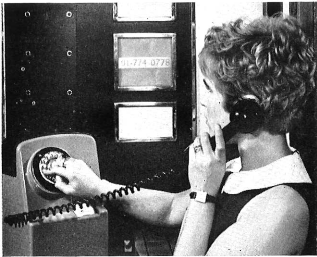
FIG. 2—Number to be dialled appears on an illuminated screen made for tests to be made both with and without the directory holders.
