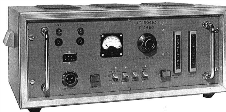
FIG. 6—Electronic group-selector tester
