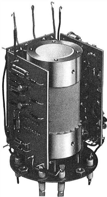
FIG. 2—Oscillator with oven and control circuits
