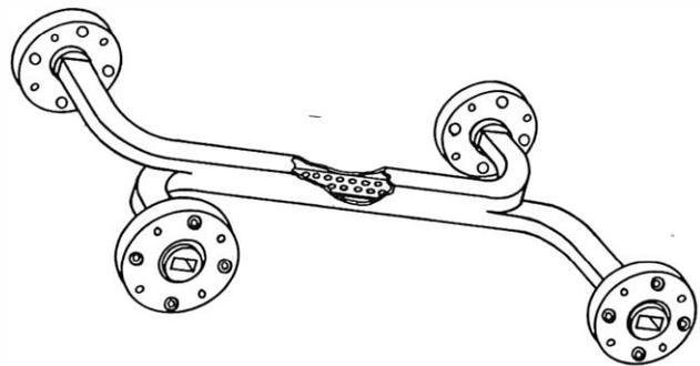
FIG. 5—Wideband coupler sectioned to show pre-drilled insert
