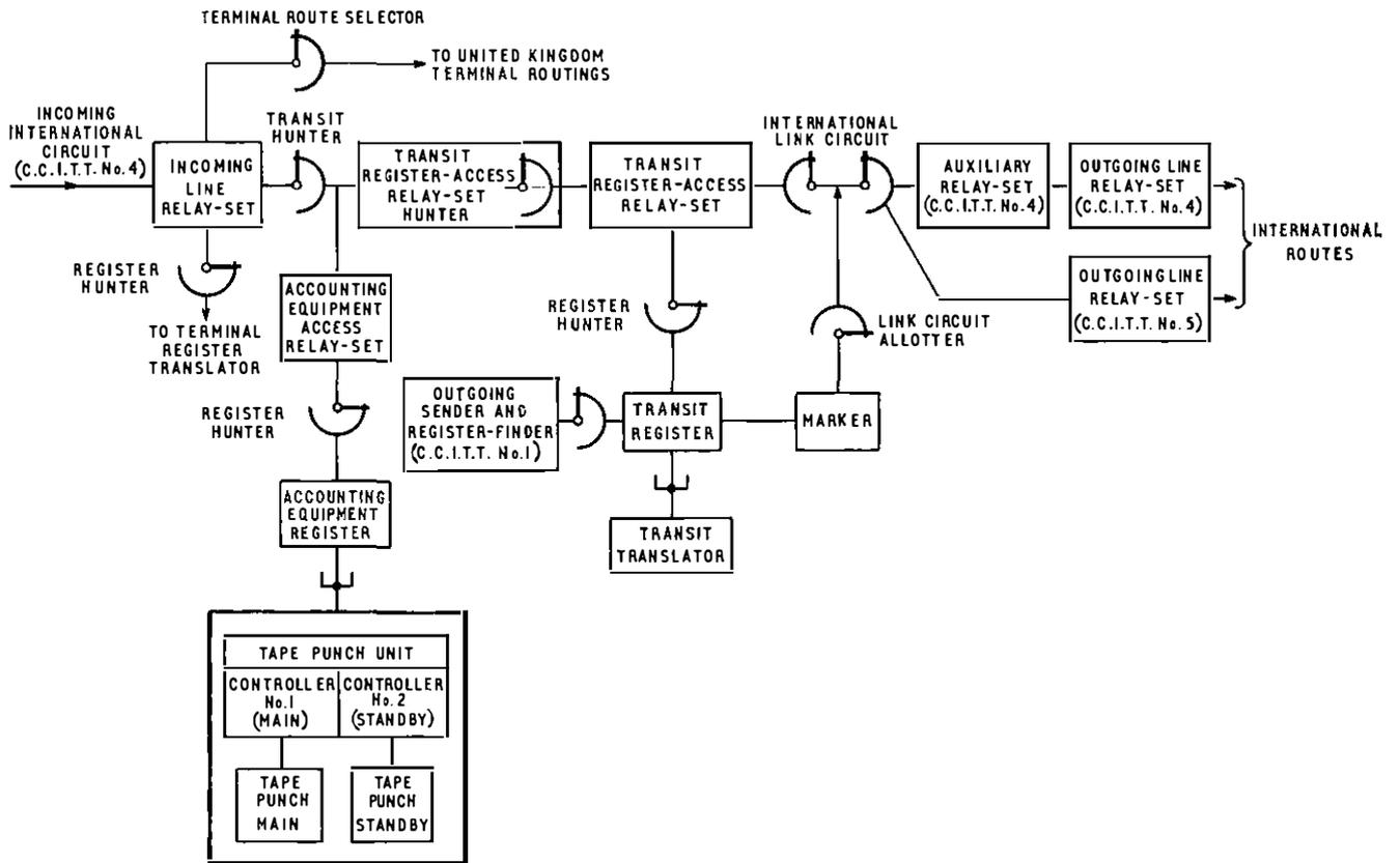
FIG. 1—Basic trunking for incoming routes using the C.C.I.T.T. No. 4 Signalling System
