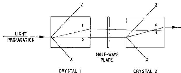
FIG. 3—A.D.P. two crystal birefringence compensation
