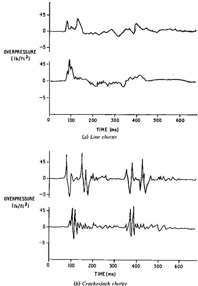
FIG. 4—Overpressure waveforms produced by simulated sonic booms
