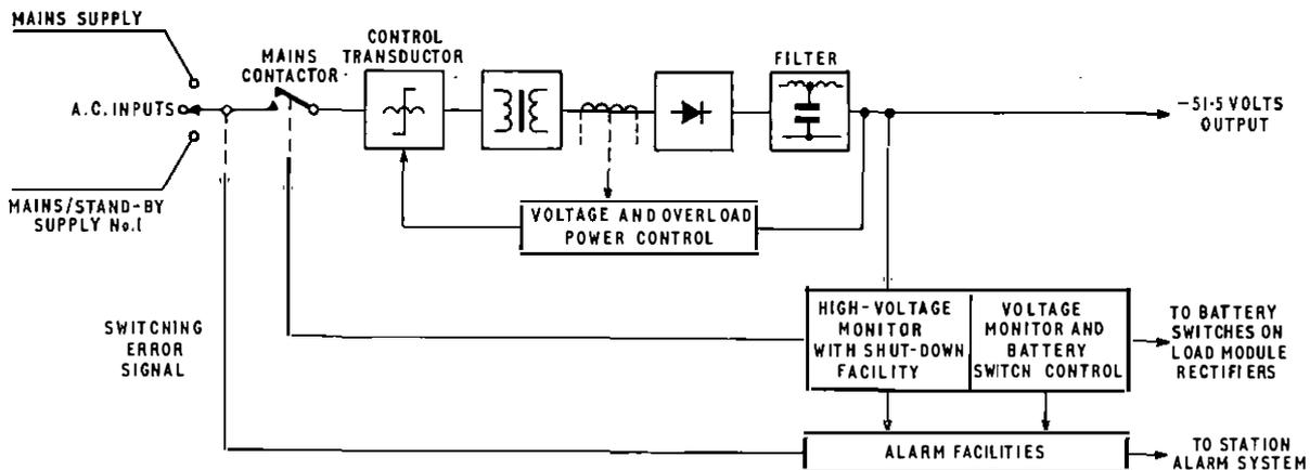
FIG. 18—Block diagram of stand-by rectifier
