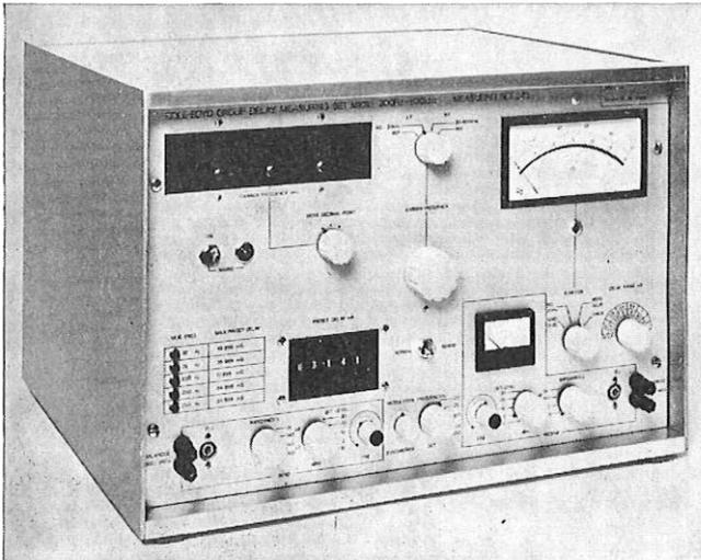
Accurate measurement is vital for dealing with **GROUP DELAY DISTORTION.** Using the COLE-BOYD Set M1010 (designated British Post Office set 37B) accurate measurements can be made at precise carrier frequency settings. End to end or midpoint circuit tests do not need a synchronising channel. The set is compatible with many other equipments. All this and much more is contained in a compact box, easily carried by one man. Send back the coupon today for our comprehensive illustrated brochure.
