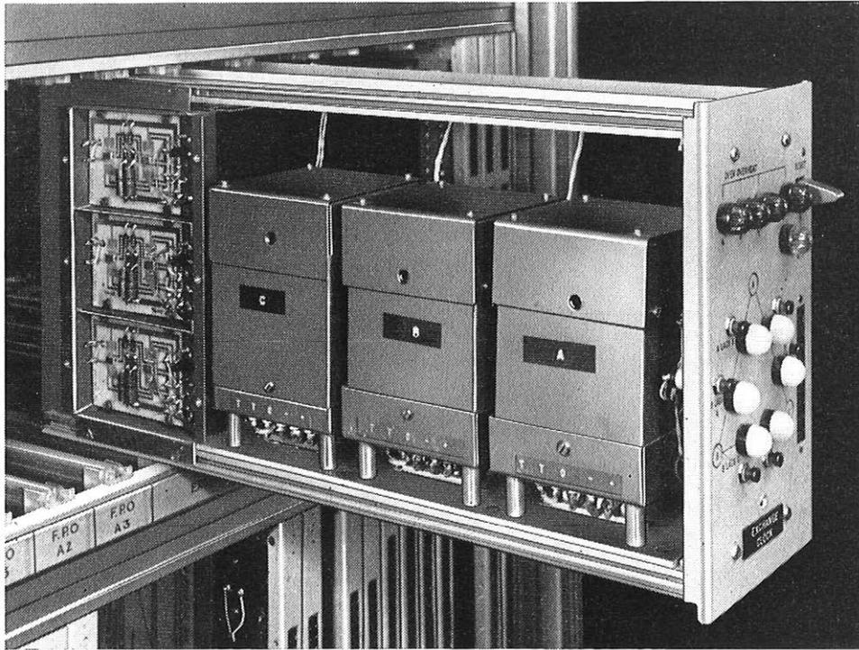
FIG. 1—Exchange clock showing oscillators and majority-decision logic circuits
