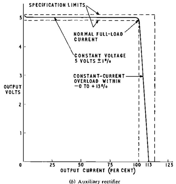
FIG. 20—Rectifier output characteristics
