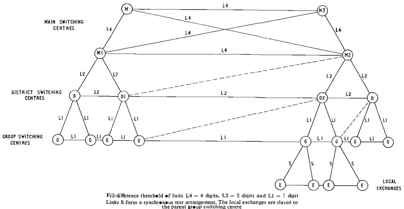
FIG. 7—Synchronization network configuration
