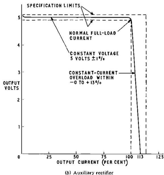
FIG. 20—Rectifier output characteristics
