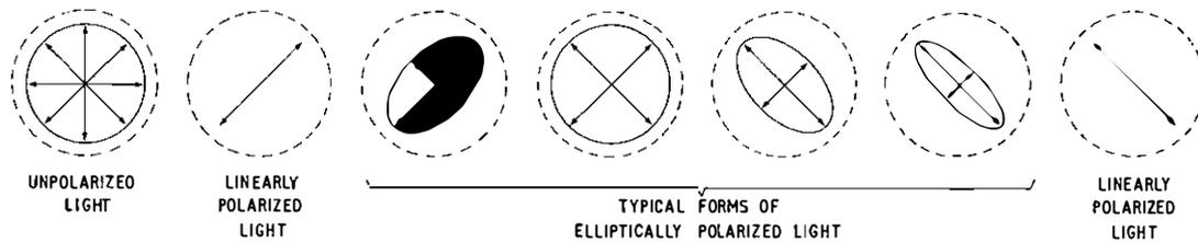
FIG. 1(b)—Elliptical polarization
