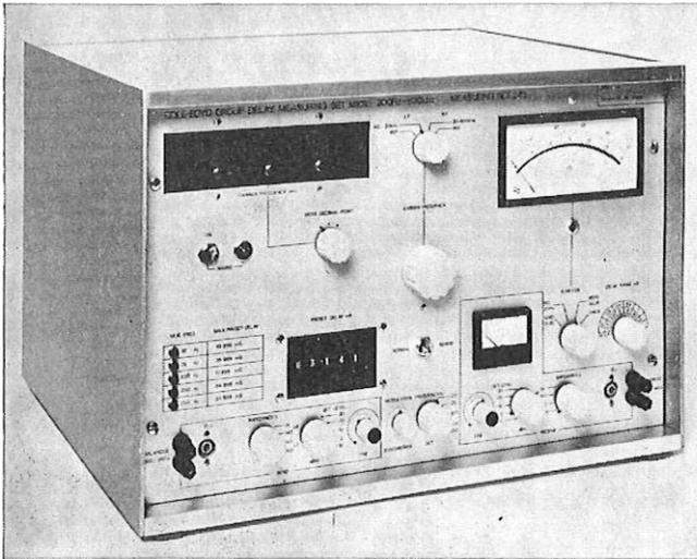
Accurate measurement is vital for dealing with **GROUP DELAY DISTORTION.** Using the COLE-BOYD Set M1010 (designated British Post Office set 37B) accurate measurements can be made at precise carrier frequency settings. End to end or midpoint circuit tests do not need a synchronising channel. The set is compatible with many other equipments. All this and much more is contained in a compact box, easily carried by one man. Send back the coupon today for our comprehensive illustrated brochure.
