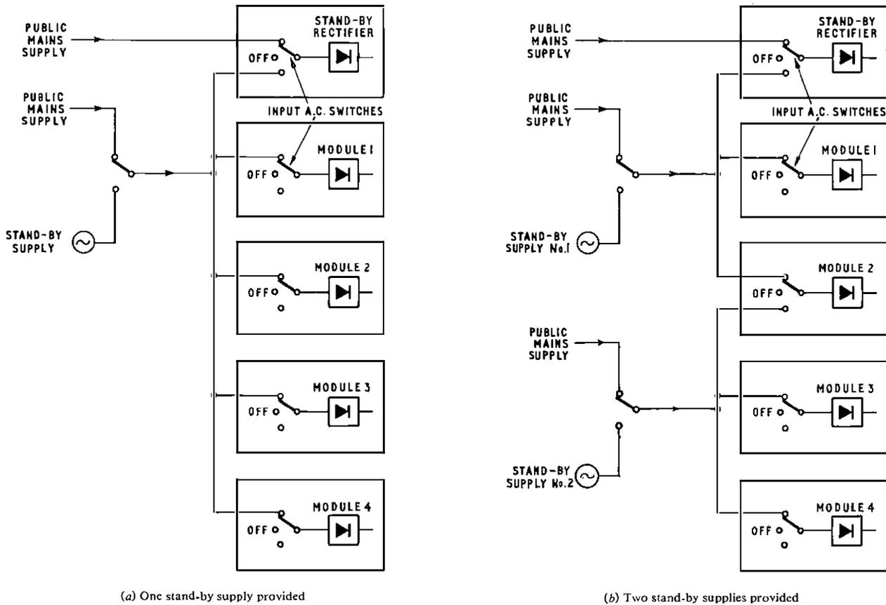
FIG. 19—Switching arrangements for a.c. stand-by supplies
