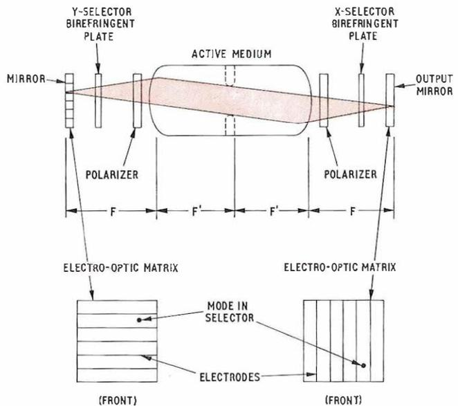
FIG. 8—Digital scanlaser with typical transverse mode illustrated
