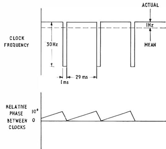
FIG. 3—Principle of clock control
