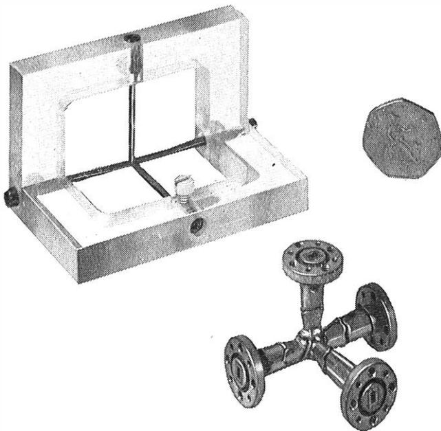
FIG. 1—Electroformed magic-tee and master
