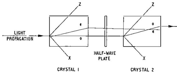
FIG. 3—A.D.P. two crystal birefringence compensation
