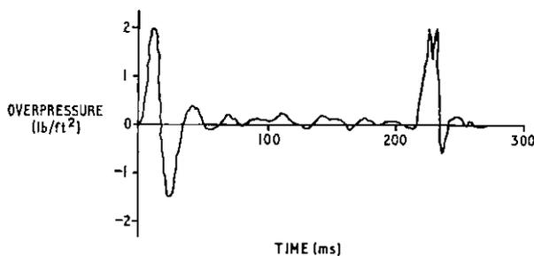
Fig. 3—Overpressure waveform generated by a *crackerjack* charge
