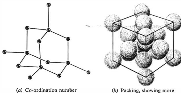
FIG. 3—Atomic lattice of diamond, silicon and germanium
