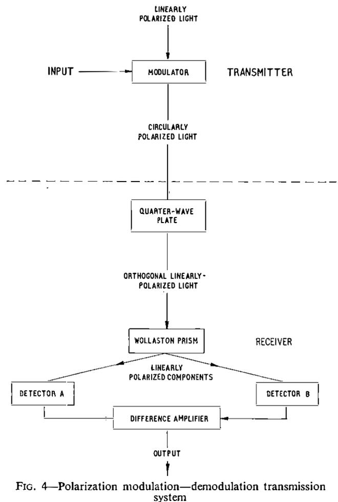
FIG. 4—Polarization modulation—demodulation transmission system
