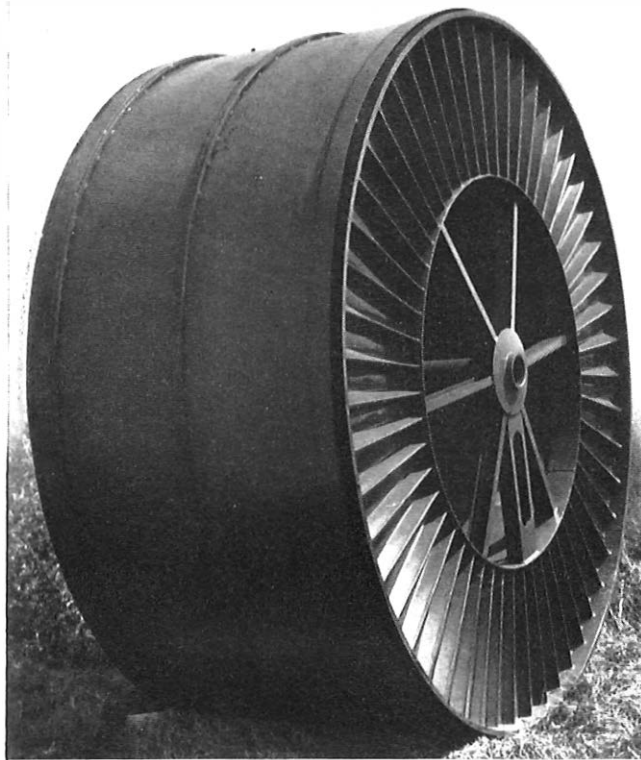
FIG. 7—Cable drum ready for transit
