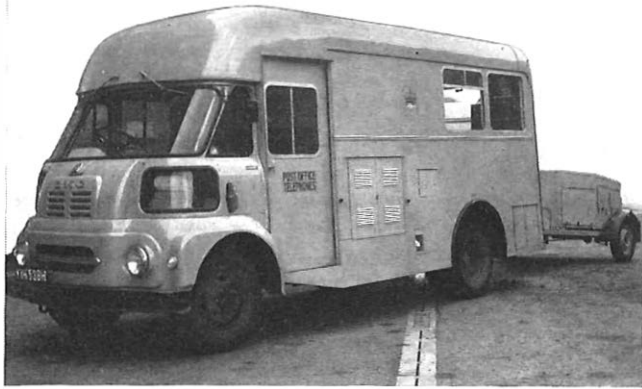
FIG. 5—New van complete with trailer generator
