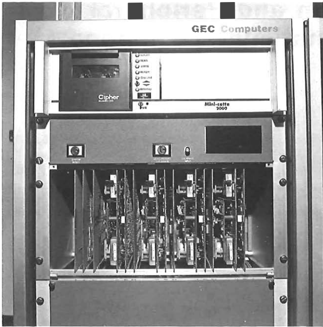
FIG. 7—Sender/receiver cards and interface cards (8 sender/receivers and 2 control boards)
