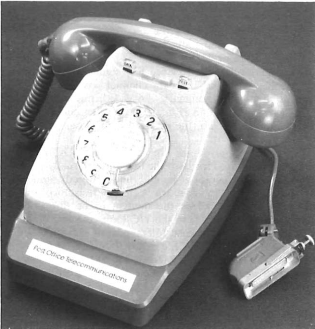
FIG. 1—Datel Modem No. 13A fitted under a telephone instrument
