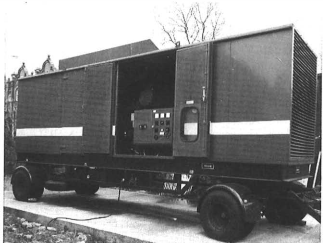
FIG. 5—Stand-by 250 kVA generator set mounted on a trailer
