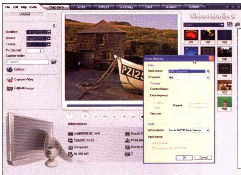
Verify that there is an output signal by connecting the player to a TV and make sure you set the video and audio sources in your capture application
