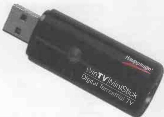
Hauppauge has expanded its range of portable TV tuners to include the WinTV-Ministick HD, a portable USB-based tuner capable of picking up local free-to-view TV channels, including those in HD. The device is no bigger than a thumb drive, with an RF port at one end to connect to an aerial. A portable mini-aerial is supplied as is the latest version of WinTV for accessing and recording channels.
