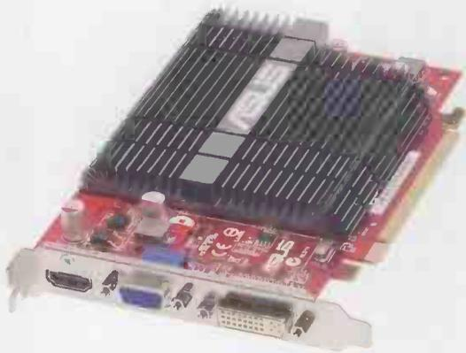
**T**he EAH4350 Silent is one of the cheapest and smallest graphics cards to arrive in our labs. It's one of the few cards to not require an additional PCI-Express power connector. Only a passive single-slot heatsink is needed to keep the chips cool, rather than a noisy fan. This makes it perfect for using in a media centre system, as it will fit into the more cramped Micro-ATX cases. It's also silent, so if you use it in a living-room PC, it won't drown out the soundtrack of your film.
