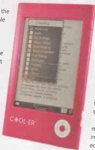
Hard controls consist of a power button on the top edge of the device, and four feature buttons down the side, including one that changes the page orientation. A navigation wheel on the front is reminiscent of the one used on iPods, but is rather heavy on the thumbs and doesn't support scrolling.
