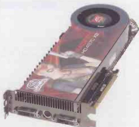
The Radeon HD 4870 X2 2G combines two 55nm 4870 GPUs into a single package. It's still the most powerful ATI graphics card available, unless a 4890 X2 is ever announced. The card has 2GB of memory, along with 1,600 shader processors (800x2). It's almost identical to two 4870s working in Crossfire, with double the number of resources available. One difference is that on most 4870 X2 cards, including this Sapphire model, an alternative interconnect between the two GPUs is available, called
