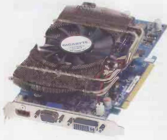
The reference clock speeds for the GTS 250 are the same as the 9800GTX, namely 738MHz for the core engine while the 128 stream processors run at 1,836MHz. As standard the card uses 512MB of GDDR3 memory, running via a 256-bit interface. Nvidia has introduced a version of the card with 1GB of memory, which runs faster than on the 512MB version, up from 1,000MHz (2,000MHz effective) to 1,100MHz (2,200MHz effective) giving the GTS 250 a memory bandwidth of 70.4Gbits/sec.
