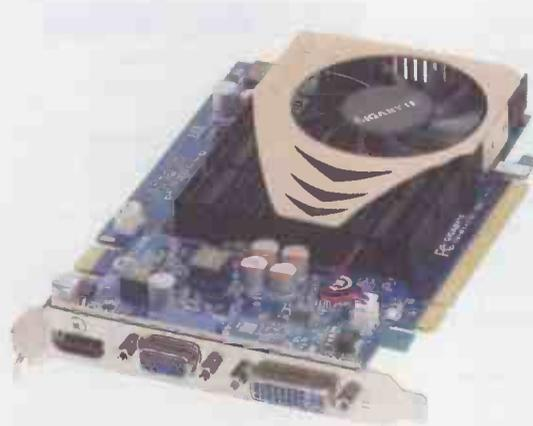
400MHz GDDR2 memory (800MHz effective) running through a 128-bit bus. This isn't nearly as impressive as the more expensive cards on test, and not well suited for modern games, even at lower resolutions.
