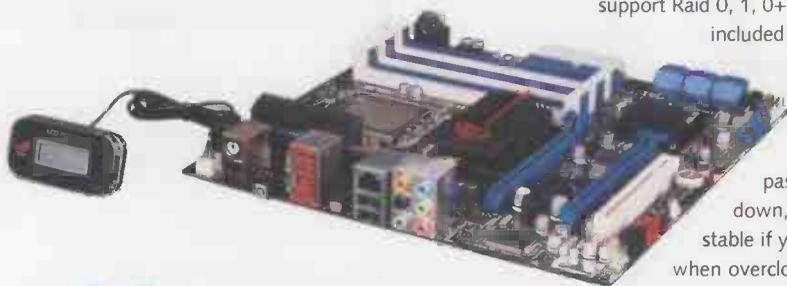
Micro-ATX motherboards aren't as popular with enthusiasts as full-sized ATX boards, as their feature set is often comparatively limited. The latest addition to Asus' Republic of Gamers family bucks this trend, as the Rampage II Gene is a Micro-ATX board built to support Intel's high-end Core i7 processors and the X58 chipset. The Gene is the most feature-rich mini-motherboard we've seen, cramming plenty of hardware into a small printed circuit board.
