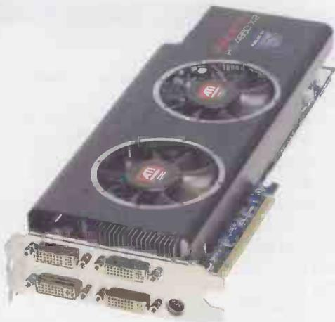
The Radeon HD4850 X2 is the second of ATI's dual-GPU cards, pairing two 4850s in a single package, with an internal Crossfire bridge. Each card is identical to those sold individually, with 1GB of local GDDR3 memory (2GB total), running at 993MHz (1,986MHz effective), with core and shader clocks running at 625MHz and a 256-bit memory interface.
