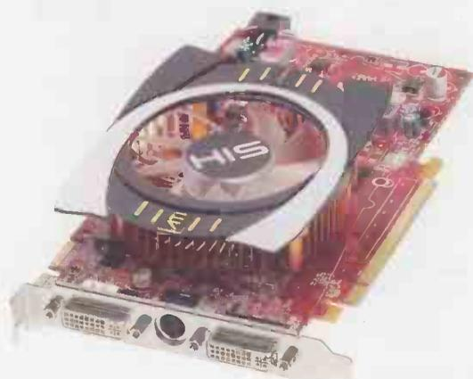
**A**lthough we received a reference ATI Radeon HD4770 board last month, the His Radeon HD4770 is a retail version. It differs from the retail board in that it has a smaller cooler design.
