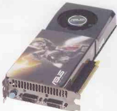
**T**he Asus Geforce ENGTX285 Ultimate Edition is a factory-overclocked version of Nvidia's Geforce GTX 285. It's a descendent of Nvidia's GTX 280, but quite a lot has changed. The Geforce GTX 285 uses the 55nm GT200b core instead of the 65nm GT200 core, and this die shrink reduces the power load (183W instead of 236W). It also allows the card to reach higher clock frequencies than the GTX 280.
