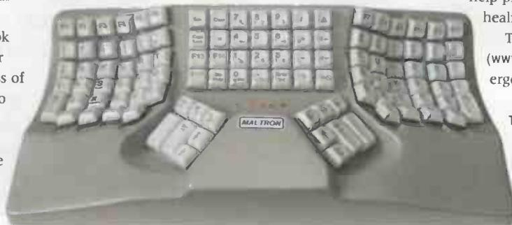
The curiously shaped Maltron L Type USB Two-handed Keyboard, is designed to keep hand and finger movement to a minimum when in use
