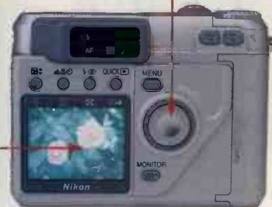
Four-way rocker switch for menu navigation
