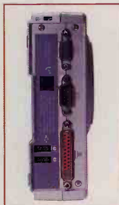
An array of ports can link the MicroPC up to a monitor, modem, printer, telephone and PDAs
