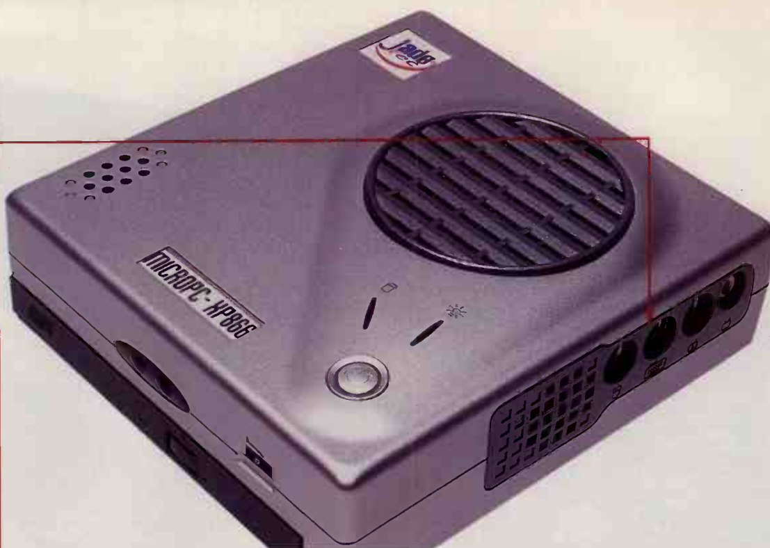
Sitting on the right-hand side of the MicroPC are AV video, S-Video, PS/2 keyboard and PS/2 mouse ports
