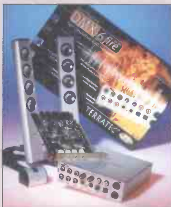
The Terratec DMX 6Fire is one of the new generation of sound cards that can do onboard 5.1 decoding
