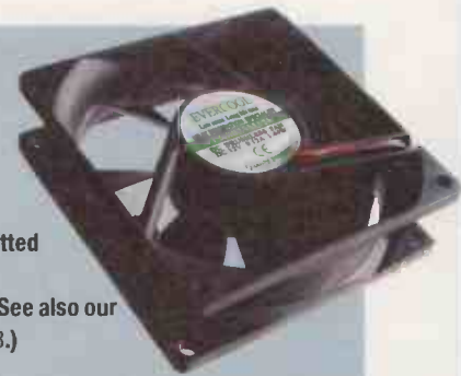
Case fans (above) and slot fans (centre) can extend the life of overheating components
