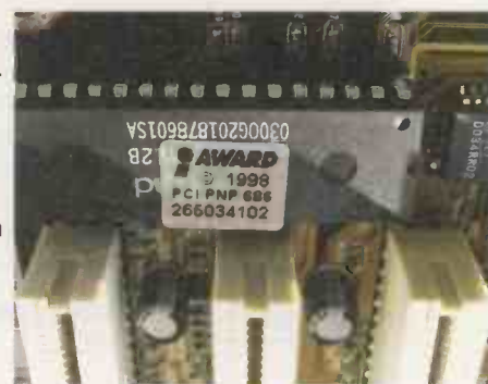
If you get into trouble, short the Jumper on the motherboard to reset the Bios
