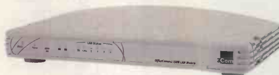
The 3Com Officeconnect Lan Modem comes with either an analogue or ISDN interface; both have a four-port Ethernet hub
