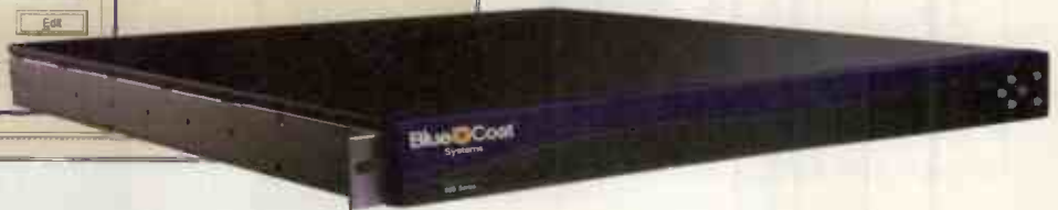
The Blue Coat SG800 Series Web Security Appliance (below) combines web caching with user authentication, content filtering and links to anti-virus scanners
