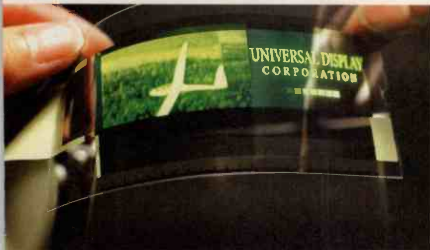
Above: Folding organic light-emitting diode (Oled) screens, will soon be used by mobile phones and PDAs
