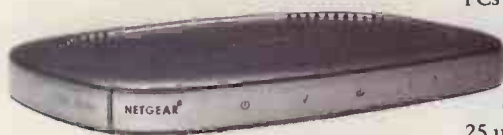
A hardware based router, such as the DG814 Platinum ADSL Router from Netgear, is a cheap and easy way of sharing a single connection to the Internet on a home or small business Lan
