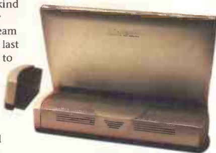
The Toshiba fuel cell, fitted to the back of a Libretto laptop. Next to it is the methanol cartridge with fuel for up to 10 hours of work
