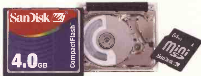
A Hitachi 4GB microdrive with its innards exposed sits between a 4GB Compact Flash card of the same size, and a 64MB mini SD card
