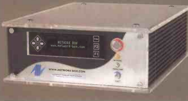
Below: Network Box appliances offer a firewall, VPN support and intrusion detection, along with anti-spam and Surfcontrol Web filtering tools
