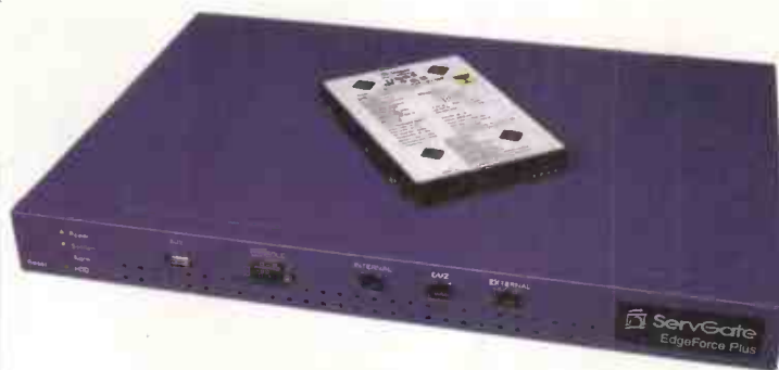
The Servgate Edgeforce is unusual as it can be enhanced using optional software and plug-in hardware modules
