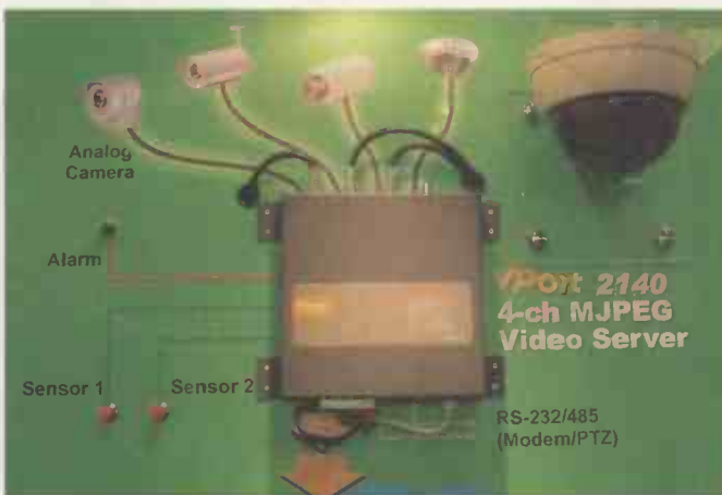
Surveillance hub supporting up to four cameras, each accessible over the web
