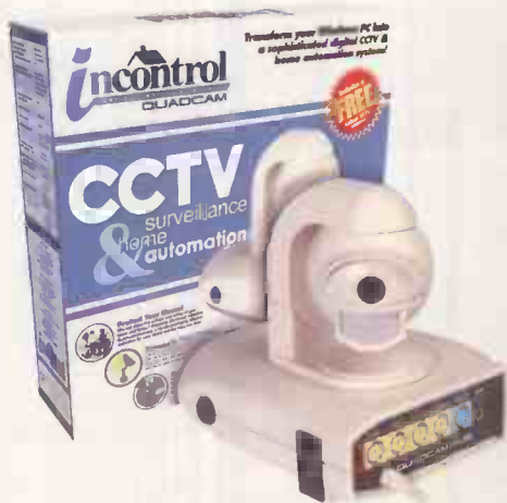
The Incontrol Quadcam system lets you monitor up to four cameras over the Internet, and can be expanded into a complete X10 home control system
