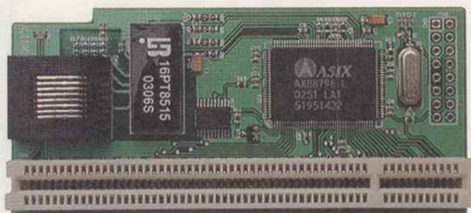
The Turbonet card equips Series 1 Tivo PVRs with an Ethernet port. You can then connect it to your PC to update settings, schedule remote recordings and even extract video
