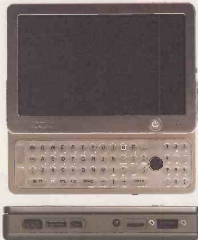
OQO's Ultra Personal Computer measures just 4.9 x 3.4 x 0.9in and weighs just under 400g, yet it runs a full version of XP on its 1GHz Crusoe processor/s. It has a 20GB hard drive, 256MB of Ram, 802.11b Wifi, Bluetooth and Firewire and USB 1.1 ports
