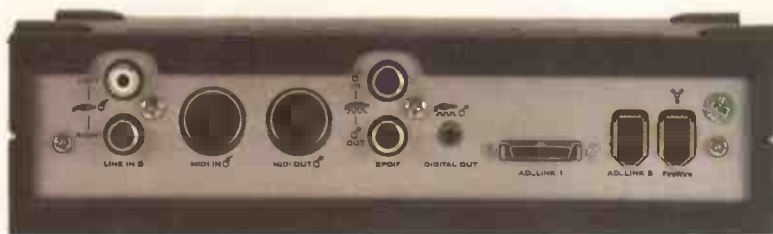
Creative's soundcards that use break out boxes generally feature full-size Midi sockets
