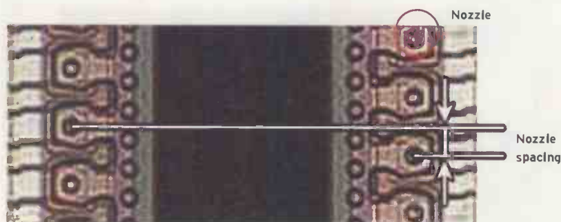
A compact arrangement allows 6,144 print nozzles to fit on the Canon i9950 print head – the printer achieves a resolution of 1,200dpi
