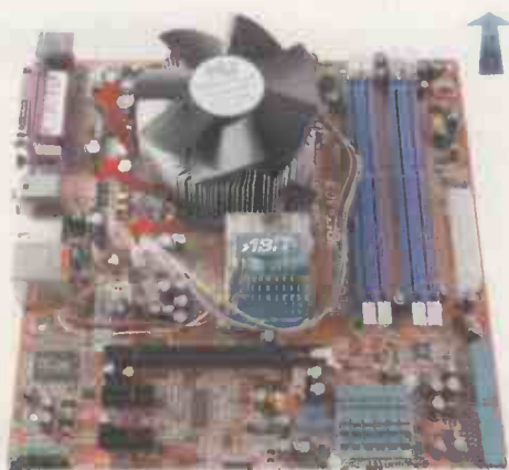
The radial construction (shown here by the Intel fan) provides extra cooling for the motherboard components (see arrows)
