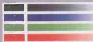
Lexmark P707: with entry-level printers the colours are visibly banded
