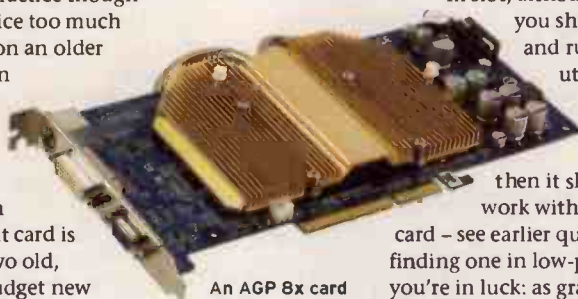
An AGP 8x card will work in a 4x slot, but it won't be running at its top speed
