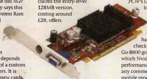
The Radeon 300 SE uses system Ram via PCI Express bus, rather than expensive onboard memory
