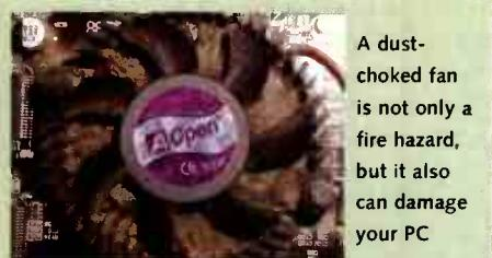
A dust-choked fan is not only a fire hazard, but it also can damage your PC
