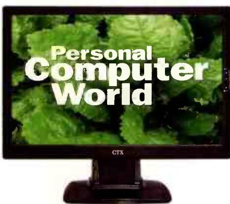
**T**he W1961A has removed all frills, and has a single analogue VGA input – therefore avoiding the tax that's put on DVI screens. There are no conveniences such as USB ports, and it's supported by a basic tilt-only stand.
