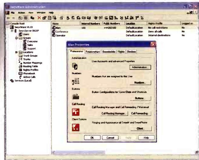
**S**wyxware is software that lets you build an IP PBX (private branch exchange) using an industry-standard PC running Microsoft Windows. A highly scalable and modular solution, we tried the new Swyxware Compact implementation – an all-in-one package, designed to give small businesses everything they need to use their own PBX.
