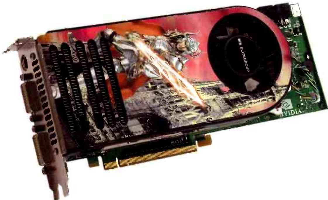
The N8800GTX-768MX is based on Nvidia's fastest processor to date, the 8800GTX. Along with the 8800GTS, this GPU is the first to support DirectX 10, a standard for Vista that improves the visuals in compliant games. The graphics card ships with two DVI-I-to-VGA dongles and both S-video and composite video leads.
