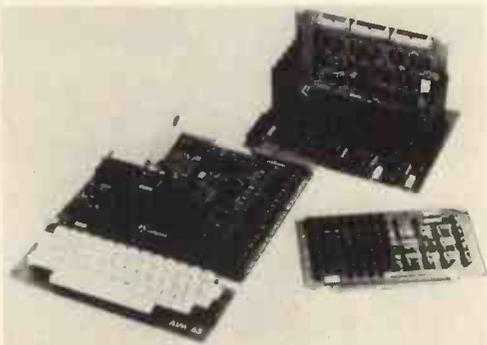
The AIM 65 expansion motherboard have five connector slots that can accommodate any of the Rockwell System 65 modules or Motorola Exorcisor modules, as well as add-on modules from Burr-Brown and other manufacturers.
