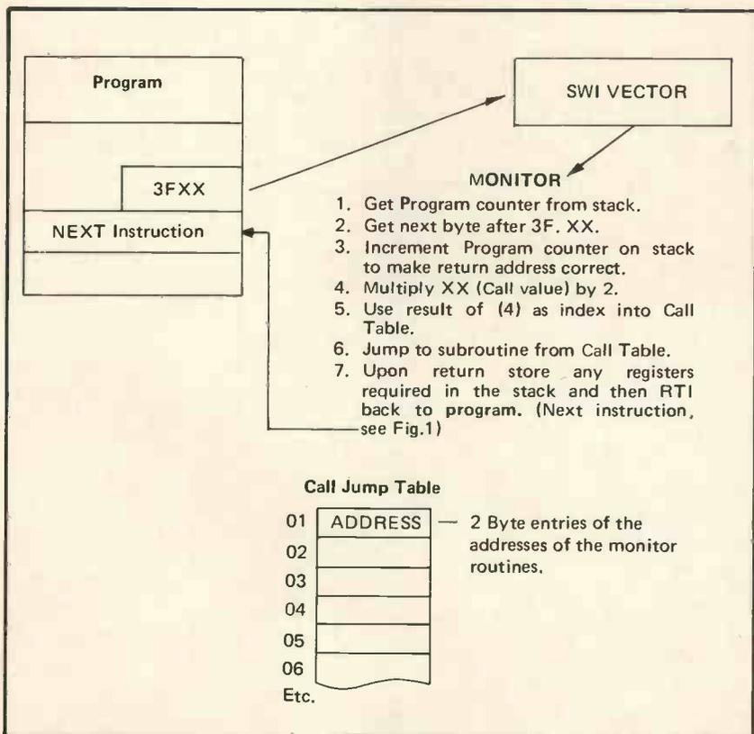
Fig. 1. Call Mechanism
