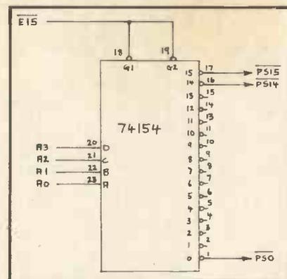
Fig. 4. Peripheral Decode
