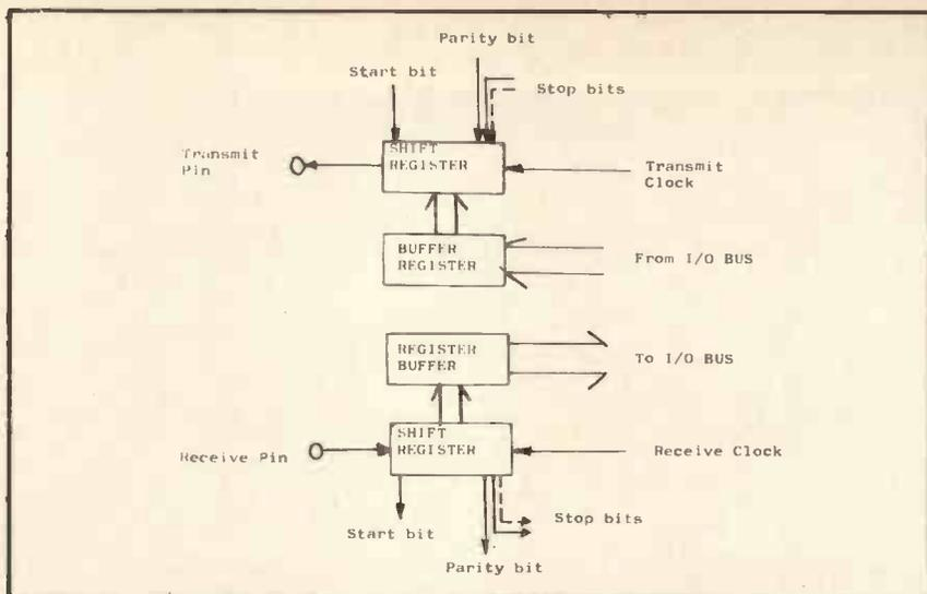
Fig. 2. Block Schematic of a Simple UART
