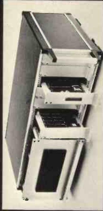
veroboard is all that is required for a full backplane, a racking system can be made available by Acorn Computers. The rack shown includes the VDU interface, two memory cards and dual floppy disc interface.
