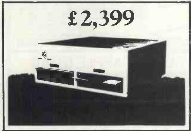
The SERIES I business/scientific computers are designed to meet the exacting needs of the small business and scientific lab markets. A Z80 ®\* disc-based microcomputer, the SERIES I is a single board computer with inherent high reliability and ease of maintenance.
