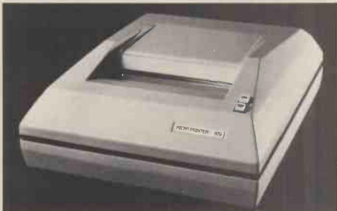
Cost of this matrix printer is £745: it prints at 120 characters per second, the head prints in both directions, it will go up to 132 columns, it is called the Micro Printerm 879. It's supplied by Leeway Data Products in Feltham, tel: 01-894 5511.
