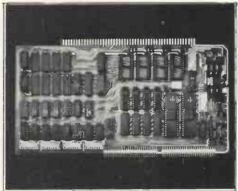
Every port is switch programmable for flexibility in interfacing various types of peripherals. Each parallel port can be switched for input or latched output. Both serial ports can be switched to any of sixteen baud rates from 110 to 19K. Each strobe and attention port flip-flop can be switched for positive or negative pulsing. The eight I/O addresses of the SWITCHBOARD can be located on any boundary divisible by eight. Price is \$199.00 kit and \$259.00 assembled retail.
