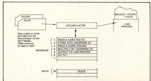
Fig. 7. A Simple Program 'Calculation of Wages'
