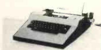
TOP QUALITY TYPESCRIPT. SOLENOID DRIVEN FOR TTL CONTROL. ROM DECODED TO ACCEPT ASCII PARALLEL DATA INPUT. 8 CPS. 11" CARRIAGE (125 CHARS)
