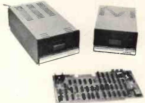
Micropolis disk drives employ higher standards of engineering to pack either 143K or 315K bytes per diskette, formatted. Supplied complete with controller card, cables, manual and software they plug directly into the S100 bus; 8080 or Z80.
