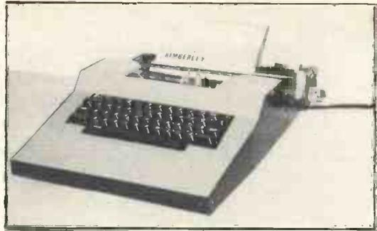
Designed for parallel data input with handshake control, ASCII coding is accepted for the 88 characters available, operating at a speed of 8 cps from a standard peripheral interface. It is supplied fully built and cased at £200 (including carriage and VAT). Alternatively, as a print mechanism only, requiring all power other than 240V, case, and TTL logic to be added, the cost is £160.
