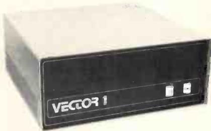
VECTOR V18A slot Motherchassis accepts the wide range of Vector S100 cards and makes an ideal base to build a microcomputer system. Computing power is available to perform a wide range of tasks from industrial control to small business.
