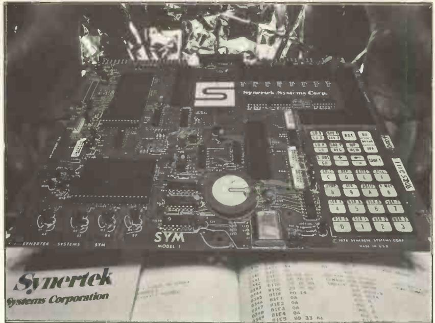
An RS232 interface permits the use of a VDU with the system and the addition of a TV/KBD interface module allows the use of a domestic TV. Again, full instructions for attaching a VDU to the system are given.
