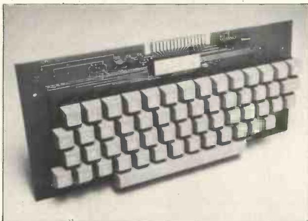
The versatile interface allows user selection of parity, positive or negative logic data and strobe outputs, alpha lock operation and both D.C. level and pulse strobe signals. A latching shift lock key is included, and all outputs are TTL-DTL-MOS compatible.
