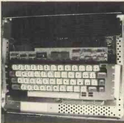
sturdy keyboard, uncluttered by any 'funny' graphics characters is more likely to suit a typist than several of the other lower priced word processing systems. On the back of the keyboard there is a socket suitable for a golfball or daisywheel typewriter.
