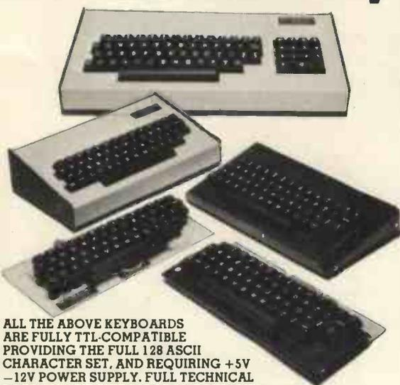
ALL THE ABOVE KEYBOARDS ARE FULLY TTL-COMPATIBLE PROVIDING THE FULL 128 ASCII CHARACTER SET, AND REQUIRING +5V -12V POWER SUPPLY. FULL TECHNICAL DATA AND CIRCUIT DIAGRAMS SUPPLIED.
