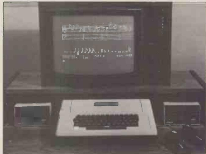
Not just a pretty picture, the music shown here. It plays, through an Apple II synthesizer card now announced in the UK by Microsense at £180 — a much lower price than I was expecting. You can attach up to three of these synthesizer cards, and each will play three notes simultaneously. Unlike the HP-85 programmable BEEP, this will emulate the sound of any instrument you care to copy; I've heard it does a very good harpsicord.
