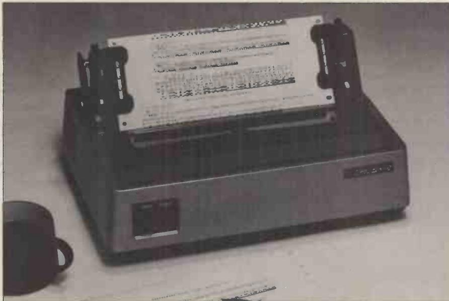
The Microline 80 offers unmatched flexibility and power for a dot matrix printer of this size, with low power consumption and low noise. The printer is of simple mechanical construction and runs without routine maintenance. The unique print head lifetime is rated to 200 million characters and can be replaced by the user. Standard half inch nylon ribbons and standard roll or fan fold paper contribute to the low operational cost of the Microline 80. Pin and friction paper feed is standard,
