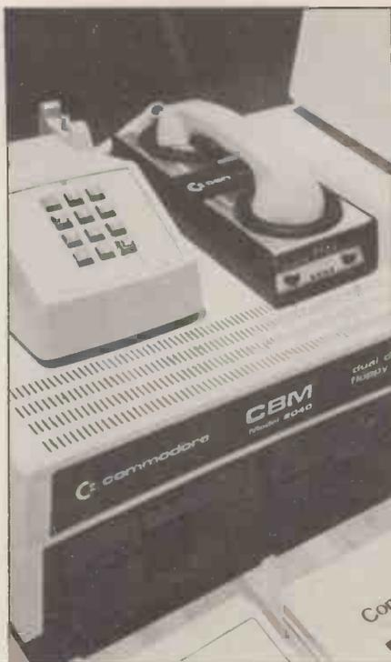
Left: Commodore's acoustic modem will let PETs converse over long distance telephone. Below: Common Sense security system — PET monitors alarm and displays security zones on screen.
