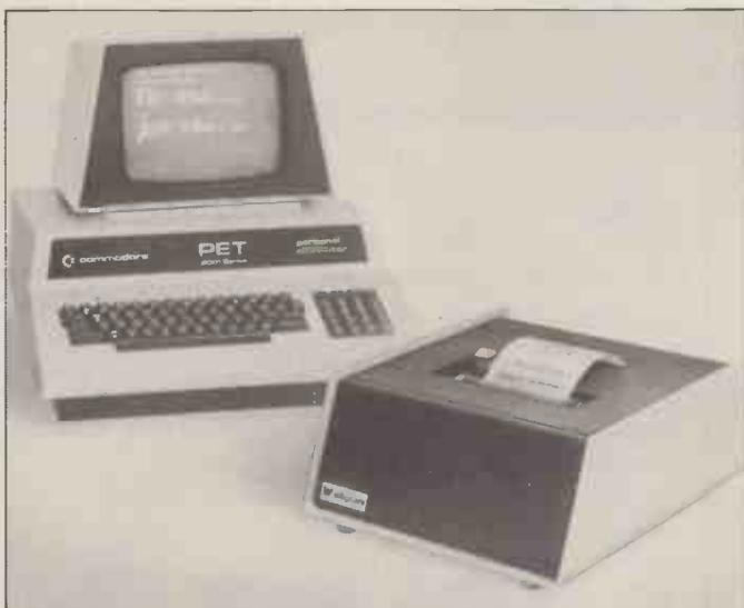
Even a very cheap print mechanism such as this tally roll printer from Whymark Instruments can get up to the £440 mark when it comes boxed and ready to plug straight into a PET. This machine prints on plain paper, so it isn't an ultra-cheap electro-sensitive arc printer (cheaper because of having no powered impact needles); it prints 40 characters per line, one line per second. Details of this and other printers and ticket preparation machines from 07372 21753.
