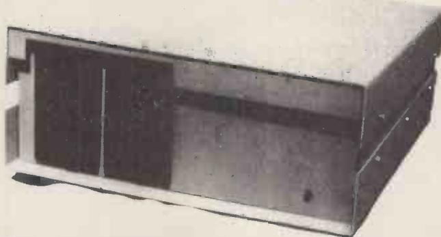
Video Interface, IEEE spec, 80 ch by 24 1, memory mapped up to 256 ch, 50Hz, £230.00
