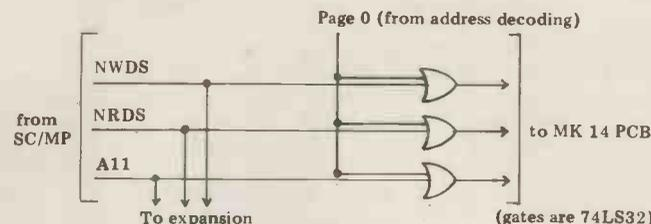
The NWDS, NRDS and A11 lines to the MK14 are ORed with the Page 0 signal (active low) so that read and write pulses are only transmitted when an access to page 0 is required; otherwise the MK14 board is effectively deselected. (Note that A11 is used as a read signal for the ROMs when low). This is a simpler solution to the problem and maintains full compatibility.
