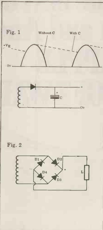
the negative half cycle of the transformer's output is not used, the half wave rectifier (as it's known) is inefficient and rarely used for high power supplies.
