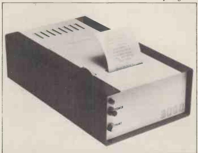
Time was when a printer using electro-sensitive paper would be sold on the basis of being cheap. This SF-30, using the electro-arc principle to vaporize aluminium and show the black paper underneath, is sold on the basis of its quiet operation and two lines-per-second operation. It's sold by Roxburgh Electronics on 079 73 3777 in Rye, Sussex.
