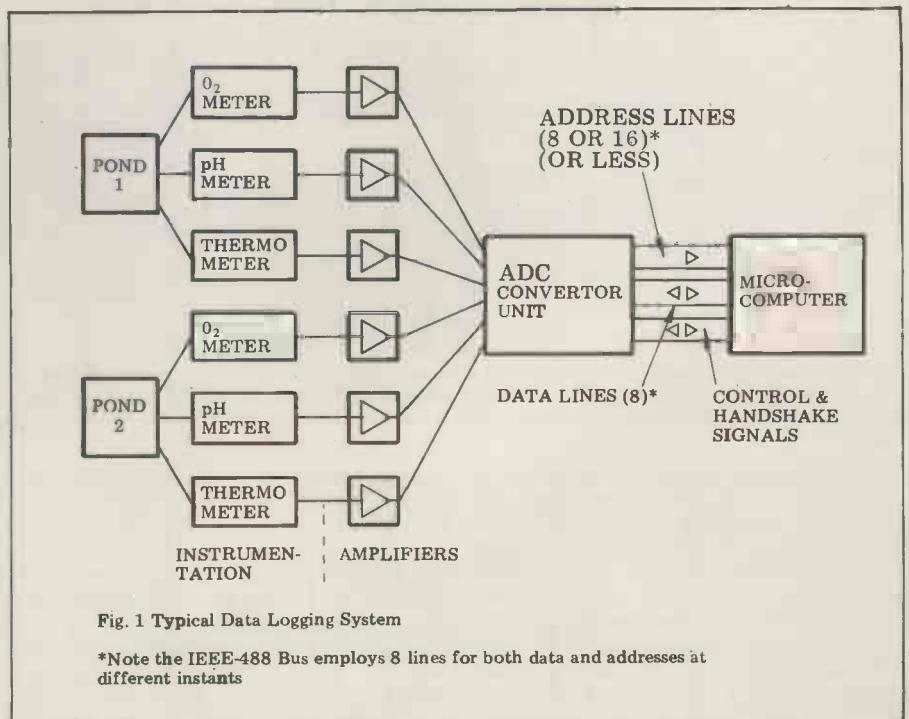
Fig. 1 Typical Data Logging System
