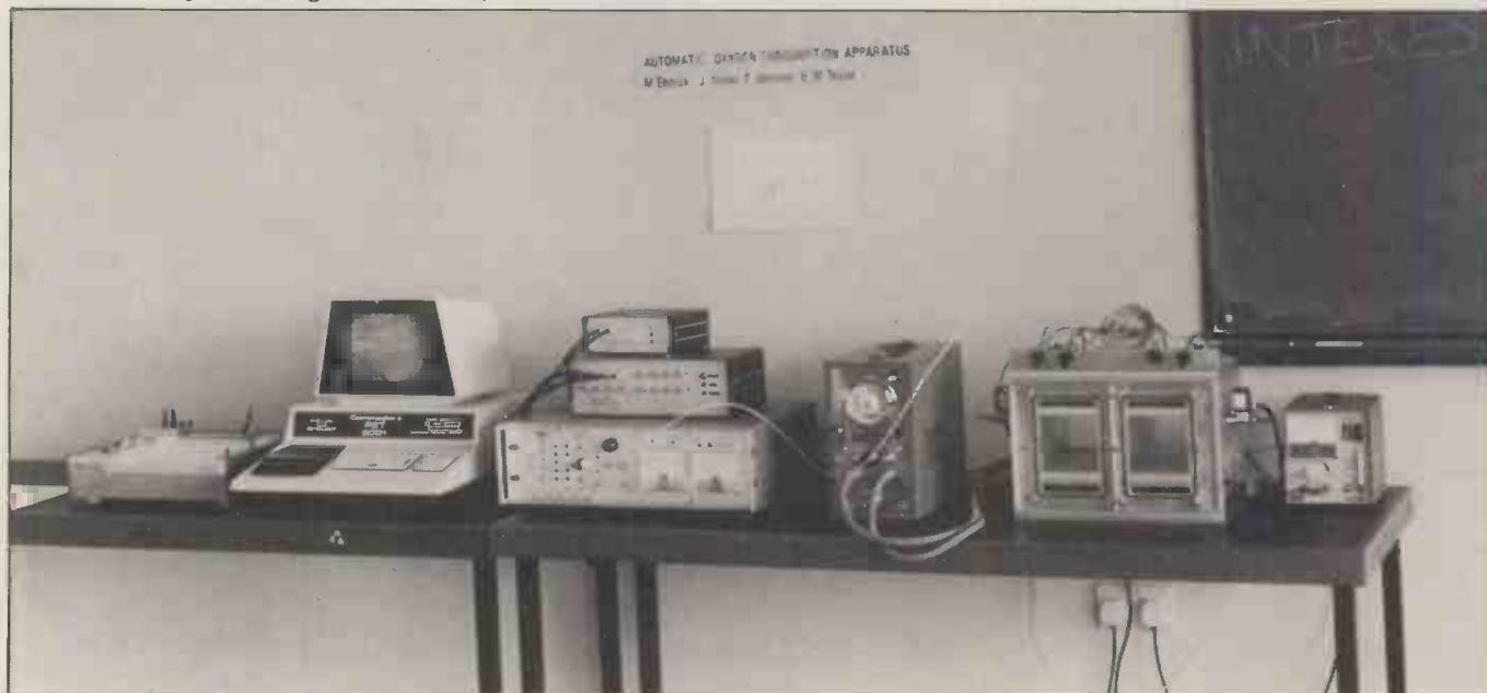
Investigating the effects of environmental temperature on metabolic rate and heat production in small newborn animals (see Fig. 5 and text). Shown are: from left to right: X-Y plotter; 16K PET; (top to bottom) 8-channel DAC unit, 16-channel ADC unit, oxygen valves controller/temperature monitor/oxygen, and CO<sub>2</sub> monitor; oxygen level monitor; dual chamber; power supply.
