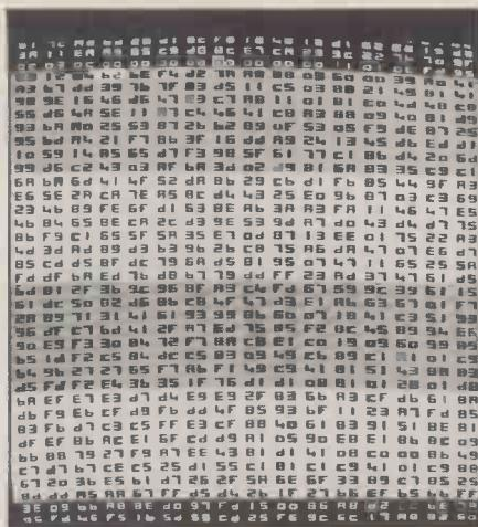
*The 512 data bytes with shaded bands of 128 bytes. The highlighted byte is the current cursor position and the status line is the line immediately above it. The other bytes in normal video are part of the scratchpad RAM.*
