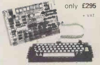
**Microprocessors** Z80A. 8 bit CPU. This will run at 4MHz but is selectable between 1/2/4 MHz. This CPU has now been generally accepted as the most powerful, 8 bit processor on the market.
