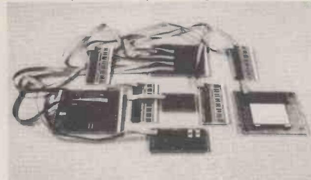
The C2 and C4 series are supported by a very wide range of expansion units, most of which plug straight into the built-in 48-line backplane. The new 16-line I/O structure uses one backplane slot (for a CA-20 or -20A) to connect with up to eight external boards. Provisional prices are:
