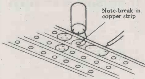
Fig 12 Veroboard underside
