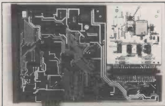
THE 8423 IS FULLY ASSEMBLED, BURNT IN AND PLUGS INTO THE 77 WAY NASBUS.
