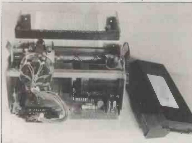
This is the new LRC M410 dot matrix printer mechanism from Impectron, which will print 40 columns at up to 120 characters a second bidirectionally onto single or multiply rolls of ordinary paper. Details on 0403 50111.
