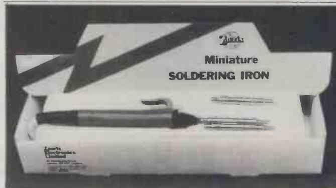
Zaerix Electronics has announced this British-made miniature soldering iron, rated at 16-18 W. The copper bit totally enclose the heating element for better heat transfer and there's a range of six bits, including a desoldering bit. There are three models, for 220/240 V, 100/110 V and 11/12 V. More on 01-727 5641.
