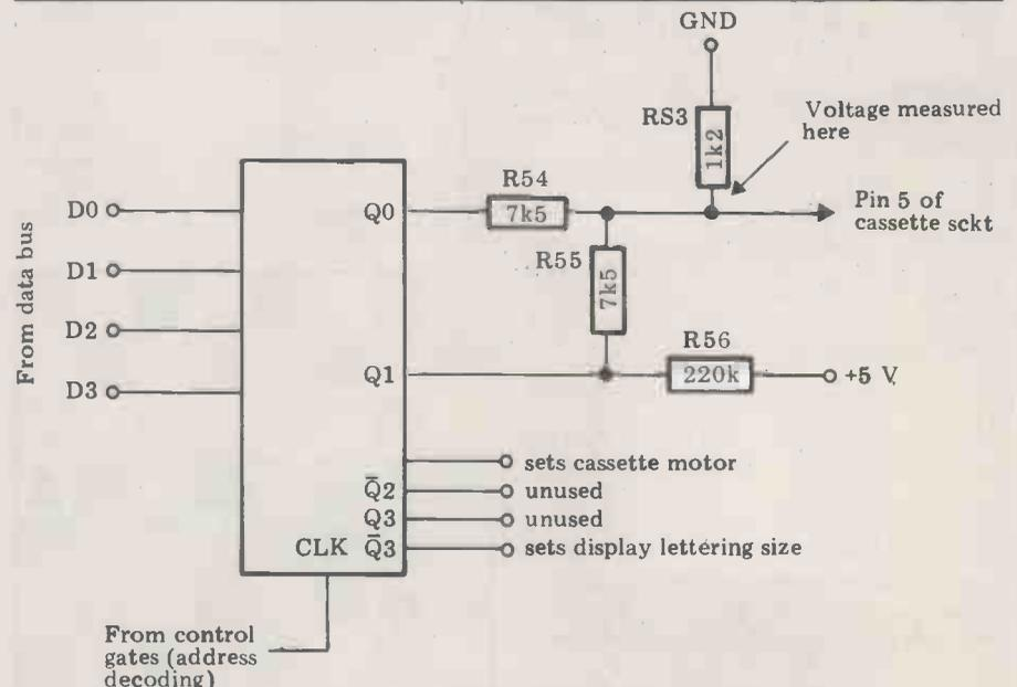
*Fig 2 The circuit of the unmodified TRS-80 cassette output latch. The cassette signal is synthesised by mixing the outputs from two sections of the latch.*
