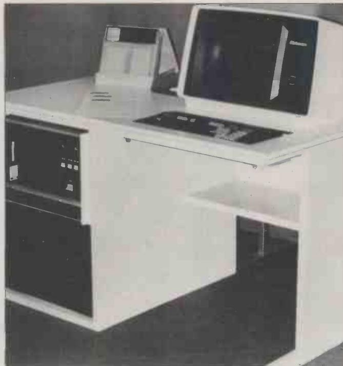
Elbit has entered the micro market with this new Z80-based system called the Micropact. It is designed to "span the complete range of distributive processing," which means it's available in configurations ranging from an intelligent transaction-processing terminal to a multi-user interactive hard disk system. Prices range from £1000 to £8000. Details on 0753 26713.
