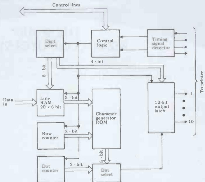
Fig 14 Block diagram of suggested control system.
