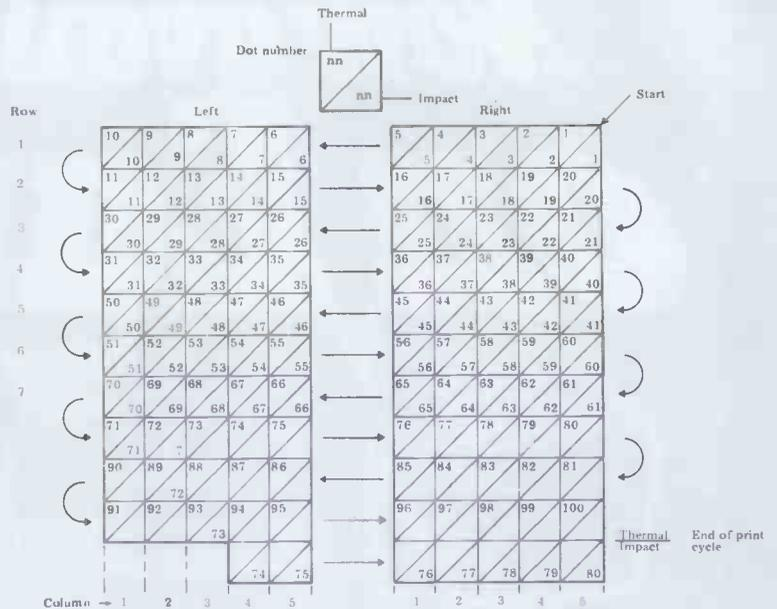
Fig 13 Character cells covered by print element.
