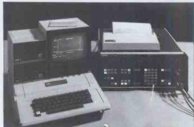
Next time some idiot tells you that micros are only toys, show him this pic. The huge black box on the right is a Solartron 1170 frequency response analyser. The most effective device which Solartron (a big company, subsidiary of Schlumberger, which owns Fairchild) could find to process the data generated by this device was an Apple II. Solartron sells the Apple as part of the data management system.
