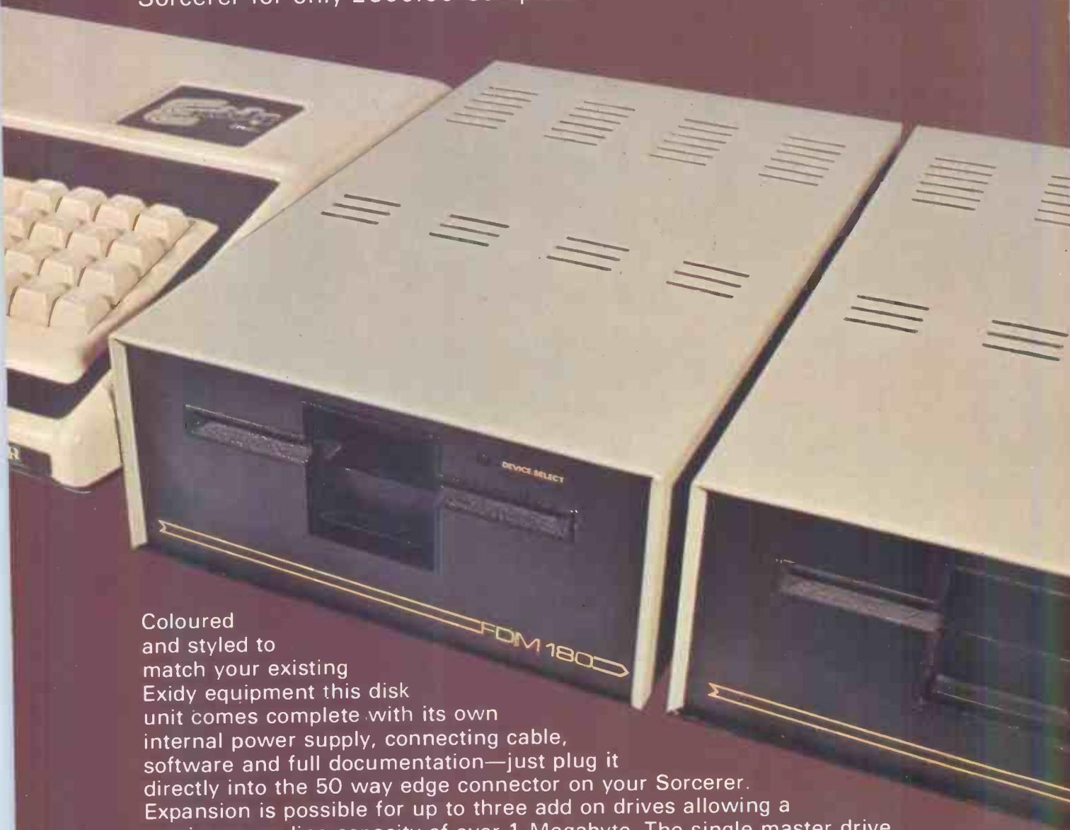
Coloured and styled to match your existing Exidy equipment this disk unit comes complete with its own internal power supply, connecting cable, software and full documentation—just plug it directly into the 50 way edge connector on your Sorcerer. Expansion is possible for up to three add on drives allowing a maximum on-line capacity of over 1 Megabyte. The single master drive will give you 315,000 bytes of formatted storage per disk.
