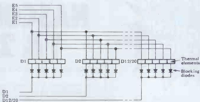
Fig 1 Electrical configuration of EPN 9112 and EPN 9120 print heads.
