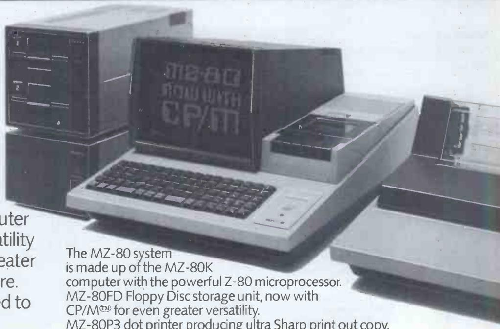
The MZ-80 system is made up of the MZ-80K computer with the powerful Z-80 microprocessor. MZ-80FD Floppy Disc storage unit, now with CP/M<sup>™</sup> for even greater versatility. MZ-80P3 dot printer producing ultra Sharp print out copy.
