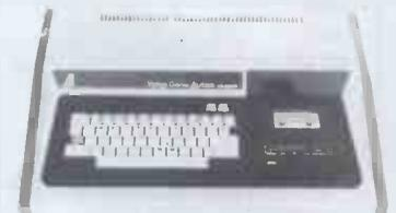
Utilises Z80, 12k level II Basic, Integral Cassette Deck, UHF O/P. 16k RAM
