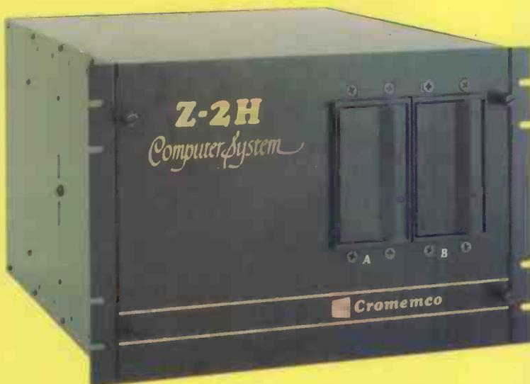
Cromemco Model Z-2H hard disc computer. 10 megabyte hard disc, 2 floppy discs, Z-80 computer and 64K memory. MicroCentre price £5,326.
