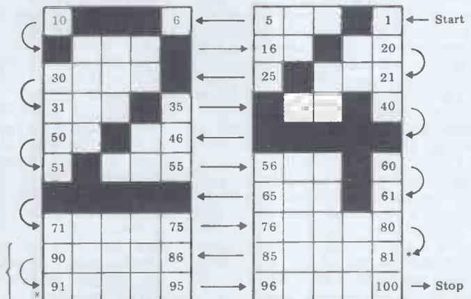
Fig 7 Print area covered by each print element.
