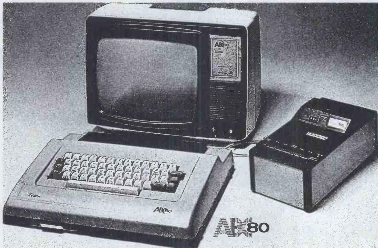
**ABC 80 - The professional microcomputer from Luxor in its basic version: display unit, keyboard and cassette tape unit.**
