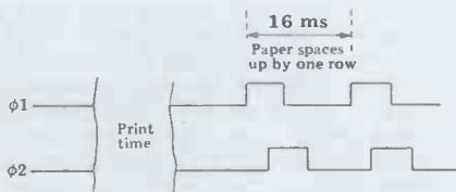
Fig 4 Suggested drive circuit and timing for stepping motor.
