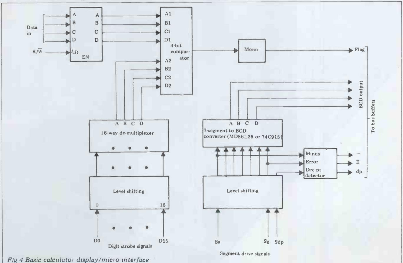
Fig 4 Basic calculator display/micro interface
