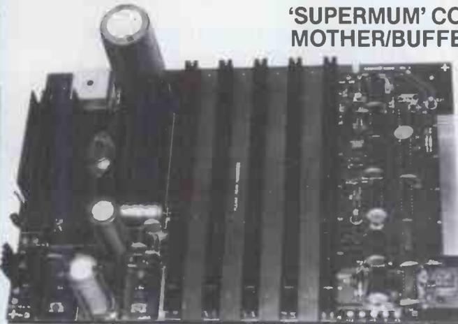
A 12 x 8 piggy-back board for the Nascom 1, it contains a five-slot motherboard, quality 5A power supply and reliable buffering with reset jump. The board facilitates easy floppy disk expansion.
