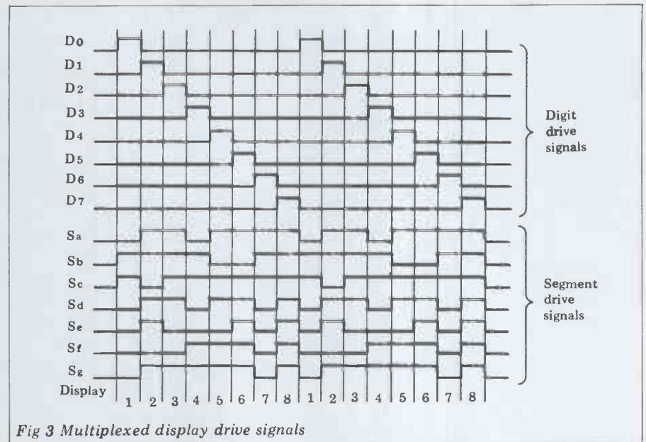
Fig 3 Multiplexed display drive signals
