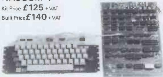
12" x 8" PCB carrying 5L SI MOS packages, 16 1K MOS memory packages and 33 TTL packages. There is on board interface for UHF or unmodulated video and cassette or teletype. The 4K memory block is assigned to the operating system, video display and EPROM option socket, leaving a 1K user RAM complete with keyboard.
