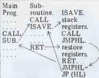
This method could be used on the Z80 and expanded to save the IX and IY registers. But, since the registers are automatically restored after the processing between the PCHL (JP (HL)) and POP PSW (POP AF) instructions, it cannot be used where the registers are needed to pass information from the
