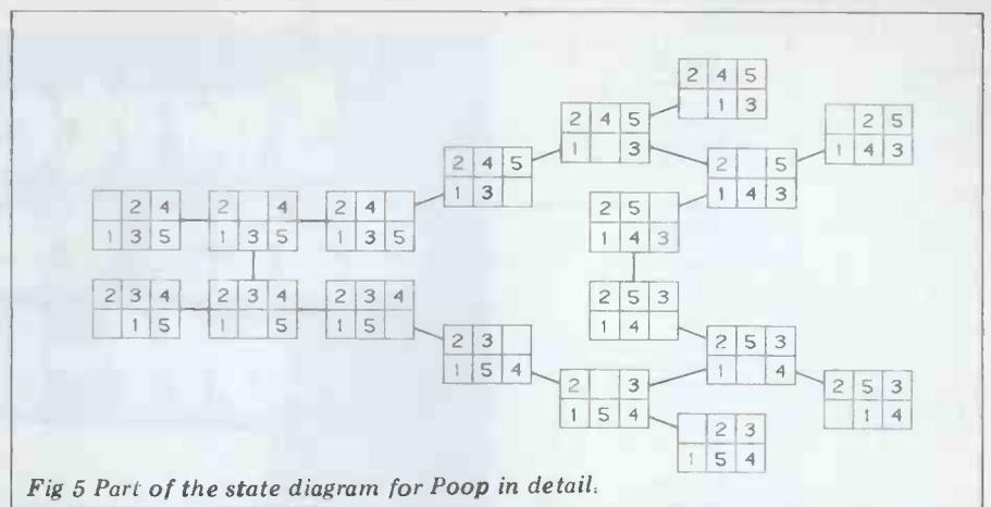
Fig 5 Part of the state diagram for Poppo in detail.
