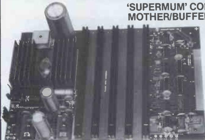
A 12 x 8 piggy-back board for the Nascom 1, it contains a five-slot motherboard, quality 5A power supply and reliable buffering with reset jump. The board facilitates easy floppy disk expansion.
