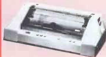
\*11x9 matrix \*High resolution graphics \*200 CPS bi-directional \*X-on/X-off \*RS232 interface \*4 print densities 10, 12.5, 15 and 16.7 chr per inch
