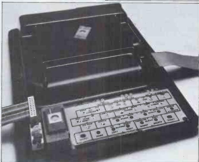
A new, improved version of the Softy EPROM programmer/development system has been launched by Barry Savage's company, Dataman Designs. As the pic shows, Softy 2 is a lot neater than the original Softy, but what you can't see just by looking is that the new one handles 2516/2716/2532/2732 single-rail (5V) EPROMs. Softy 1, which handles 2708 and 2716 three-rail EPROMs, is still available, by the way. More on 0305 68066.
