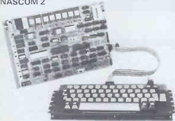
Kit includes all parts to build CPU board which has resident 8K Microsoft BASIC and 2K NAS-SYS 1 monitor for machine code programming. Included with kit is a fully assembled LICON QWERTY SOLID STATE KEYBOARD specially designed to exploit the potential of the NAS-SYS monitor. Other interfaces include video to monitor or domestic TV, Kansas City standard cassette interface (300/1200 baud) or RS232/20mA teletype interface and two uncommitted parallel ports.
