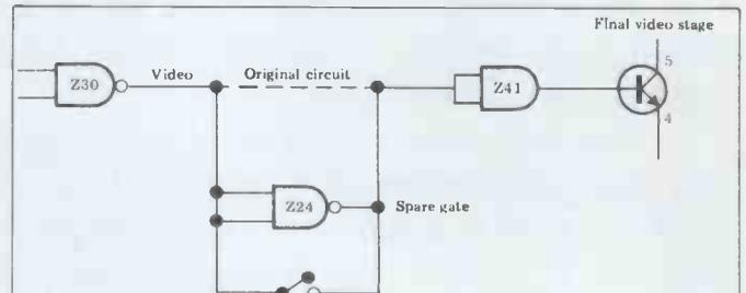
Fig 1 Logic diagram for TRS-80 reverse video mod.
