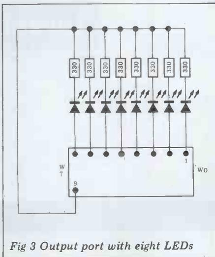
Fig 3 Output port with eight LEDs
