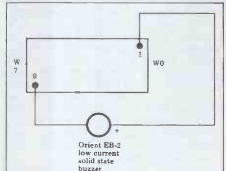
Fig 6 Output port driving solid state buzzer on chan 0.
