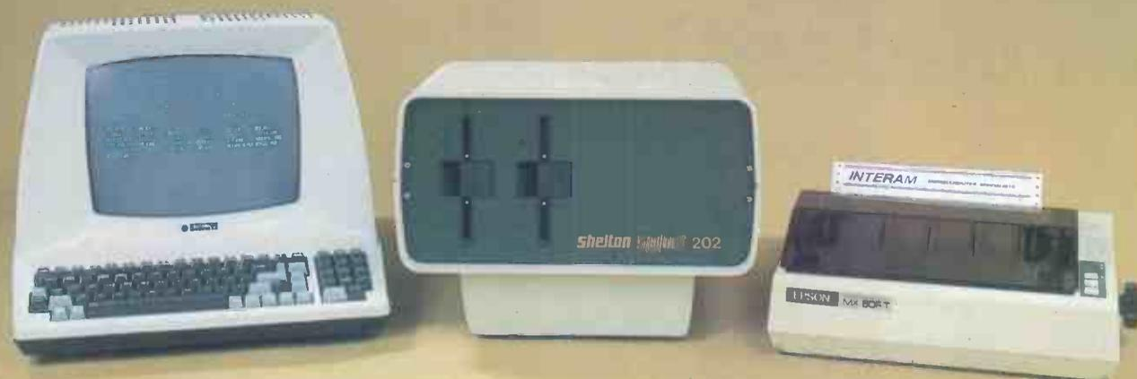
**SIG/NET 202S – Z80A CPU, 64K RAM, 2 FAST STEPPING 5¼" DRIVES (400K, Superbrain compatible format), 2 SERIAL RS232 PORTS, CP/M 2.2**
