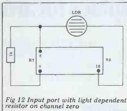
Fig 12 Input port with light dependent resistor on channel zero
