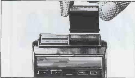
**Snap-in more memory.** A single module will double the memory available. A quad module adds no fewer than 256 registers at once. Suddenly you've over 1800 lines of memory at your command.
