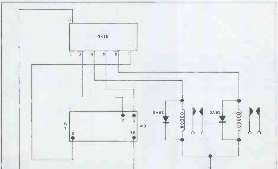
Fig 5 Output port driving two relays using 7416 inverting driver.
