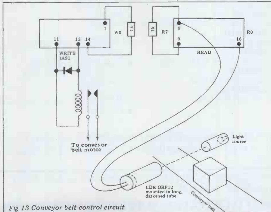
Fig 13 Conveyor belt control circuit
