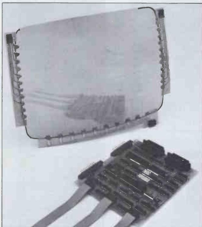
All the fiddly bits around this naked screen are designed to see if a finger is touching the glass. The idea is that a computer can detect where on the screen someone is pointing and then check what it has displayed at that spot.
