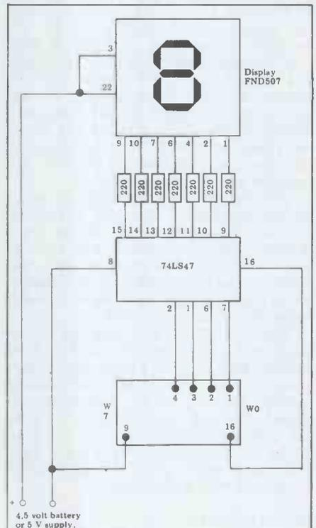
Fig 7 Output port driving single seven-segment display on channels 0-3
