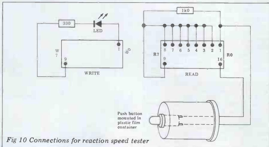
Fig 10 Connections for reaction speed tester
