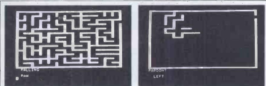
Fig 2. The Dragon demonstration program. (a) As supplied, the walls become visible only when the player bumps into them. (b) A version modified to leave the maze in view. The player steers towards the exit by spoken commands up/down/left/right, trying to evade the dragon. The last two commands spoken remain in
