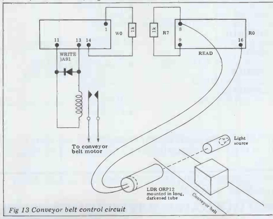
Fig 13 Conveyor belt control circuit
