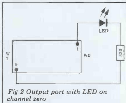
Fig 2 Output port with LED on channel zero
