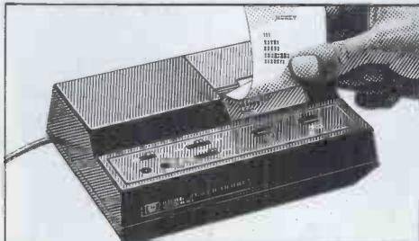
**Plug-in a printer.** The HP-41C printer handles upper and lower case, in alpha, numeric and graph-plotting modes. Use it for final hard copy, or to follow program execution.
