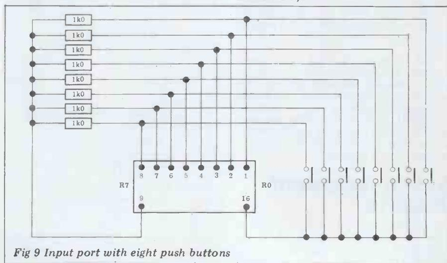
Fig 9 Input port with eight push buttons
