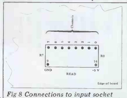
Fig 8 Connections to input socket
