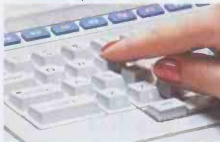
A typewriter-style keyboard incorporates characters and symbols plus a numeric key-pad and ten user-definable keys for fast and simple operation.
