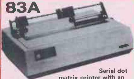
Serial dot matrix printer with an impressive list of features including: 136 cols, 120 cps bidirectional, short line seeking, graphics, dual interfaces, 96 ASCII
