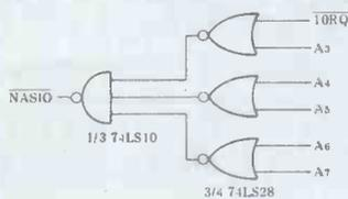
NASIO is now pulled low when a port used by the Nascom 2 is selected, as desired. NASIO can then be safely ignored on all expansion boards and ALL 256 ports can be uniquely addressed (unlike the partial decoding done on, say, the Gemini EPROM board and others).
