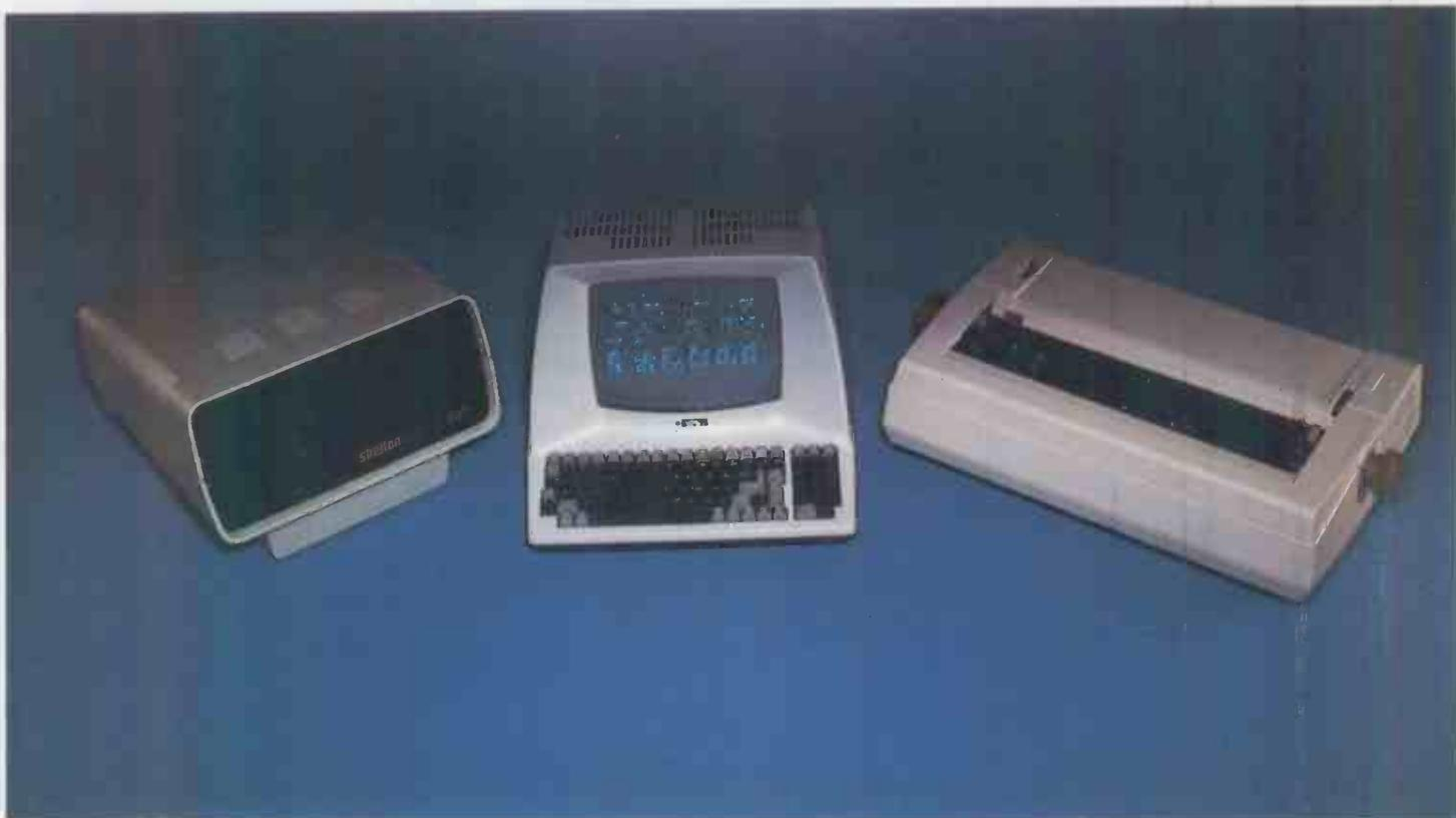
The SIG/NET 202S is a high performance computer based on a 64K, Z80A CPU-RAM module and uses the CP/M operating system. A floppy disk controller handles the popular, fast stepping, Tandon disk drives. The SIG/NET comes with a programmable, dual RS232 serial interface module. Multi-user and network configurations are possible and with the addition of a hard disk make the SIG/NET range very powerful.
