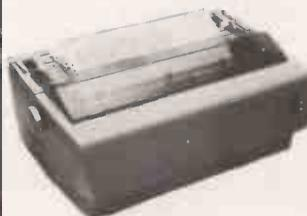
Bi-direction. 25 cps. Low cost supplies. Standard Daisy Wheel. Carbon and fabric ribbons. Parallel or RS232 interface. Sheet feeder options.
