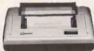
High throughput. 180 cps. Bi-direction. Fast head travel. Space skip over. Lower case descenders. Enlarged and bold fonts. Parallel RS232 and current loop interfaces. X on X off. Condensed character option. Sound reducing option.
