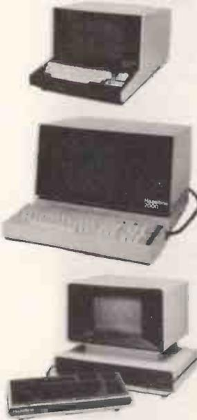
H1000 The low, low priced teletypewriter-compatible video display terminal, offering your choice of transmission speeds up to 9600 baud as well as parity generation and checking. 12x80 display upper case ASCII, RS232 interface, choice of baud rates Standard baud rates either (a) 110/300 or (b) 300/1200. (£25 surcharge for other combinations up to 9600 baud).
