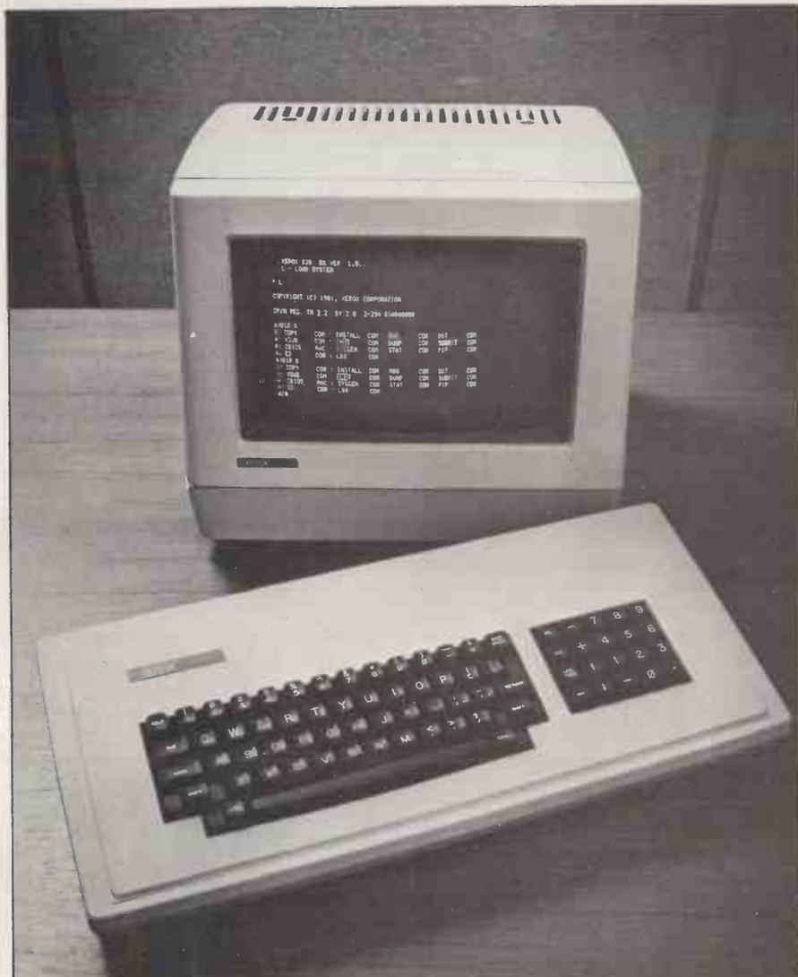
Dubbed 'The Worm' (an allusion to the success of the Apple II), the 820 is the Xerox entry to the personal computer market. Built around well-tried components like the Z80 CPU, there is nothing radical about this system; instead, it is a solid, no-frills computer with virtually no software included in the price.
