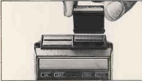
**Snap-in more memory.** A single module will double the memory available. A quad module adds no fewer than 256 registers at once. Suddenly you've got over 1800 lines of memory at your command.
