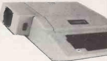
Heat is hardware's greatest enemy. The APPLE II's design provides insufficient ventilation for peripheral cards. If you use several, the results could be disastrous. Cool your APPLE with the SUPER FAN II.
