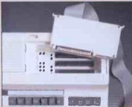
*Above: machine has three slots for plug-in modules. Below: interior features densely-packed PCB.*
