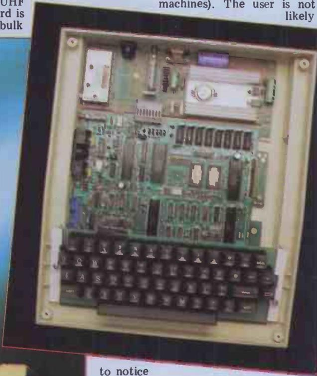
to notice any difference over a 6502 based machine but the efficient instruction set of the 6809 should help in squeezing as much code as possible into a restricted memory space and should give speed advantages, while being similar enough to the 6502 to make translation of software a reasonably straightforward task.
