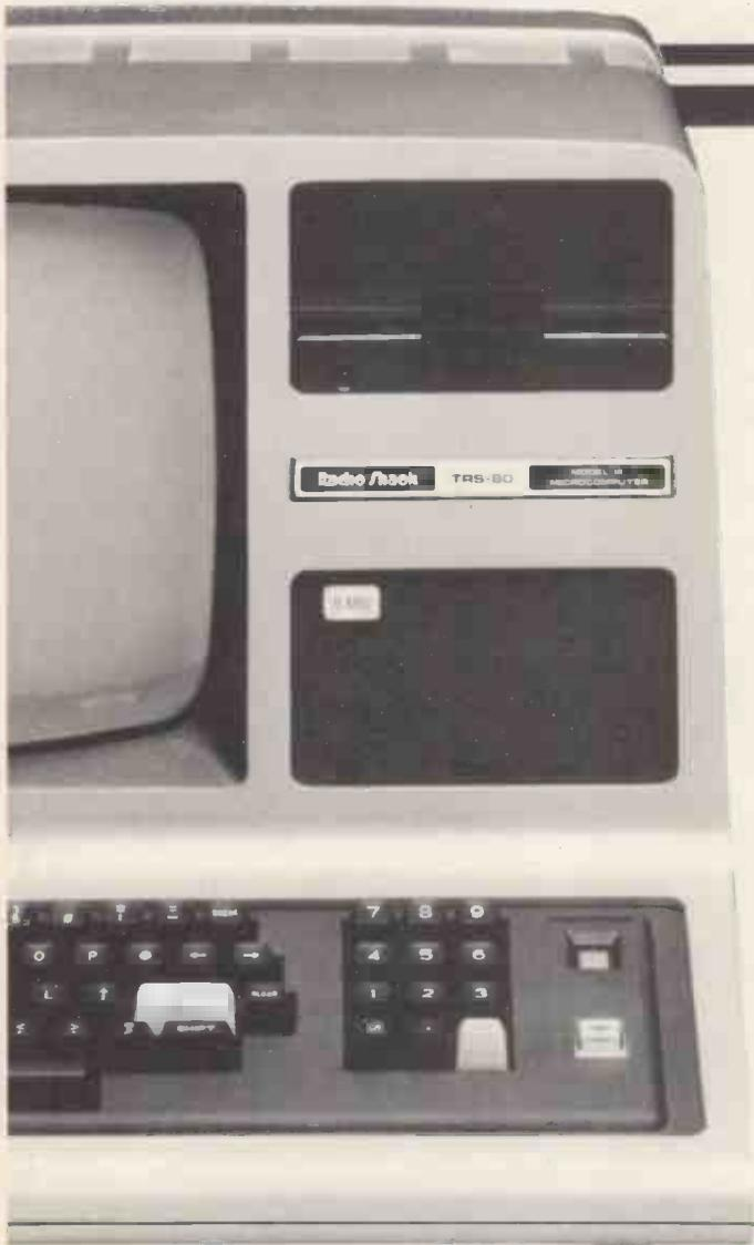
With the quality Rodime R0200 Series of 5¼" Winchester Drives Cumana gives TRS-80 Model III owners high capacity at low cost. Internally mounted hard disks offer storage capacities from 5.25 M.B. to 21 M.B. The internal kit is comprised of mounting frame, hard disk, power supply unit, controller and fan.
