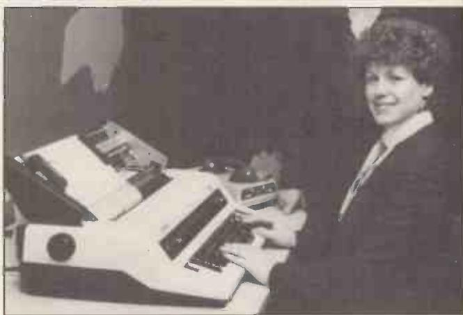
The typewriter in this picture is a computer. It is the Olympia ESW 103 KSR, and KSR stands for Keyboard Send Receive - which means it can be used as a terminal to a remote computer.
