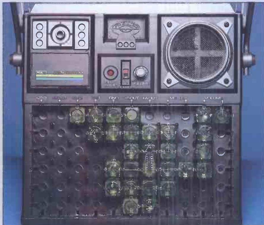
The plastic lid lifts up to allow the user access to the computer panel and the electronic components
