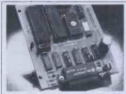
FOR EPSON PRINTERS, Microbuffer/E comes in two serial versions — 8K or 16K (upgradable to 32K) — and two parallel versions — 16K or 32K (upgradable to 64K). The serial buffer supports both hardware handshaking and XON-XOFF software handshaking at baud rates up to 19,200. Both interfaces are compatible with standard Epson commands, including GRAFTRAX-80 and GRAFTRAX-80+. Prices range from \$159 to \$279.
