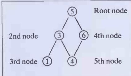
You have now created a 'sort tree' and at a first glance you may well be wondering what use such a structure can be. It can be noticed that the leftmost item on the tree is in fact the one with the lowest value. It is also apparent that the rightmost item is in fact the one with the largest value. Other than that there does not appear to be anything special about the arrangement.
