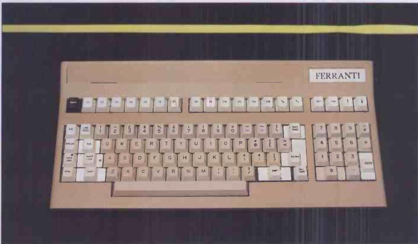
*The function keys offer a combination of twenty six programmable functions which are used effectively in applications programs.*
