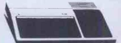
This microcomputer is based on TMS9900 16-bit microprocessor. It includes 16K RAM, 16 colour high resolution graphics (192 x 256). The screen display is 32 characters, 24 lines TI-BASIC. Full-size keyboard. For Software there are about 1000 programs to choose from. There are a lot of peripherals available, e.g. Disk Drives, Disk Interface, Speech Synthesizer, Extra RAM, Additional Language (PASCAL, TI-LOGO, ASSEMBLER).
