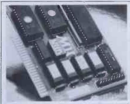
FOR APPLE II COMPUTERS, Microbuffer II features on-board firmware for text formatting and advanced graphics dump routines. Both serial and parallel versions
