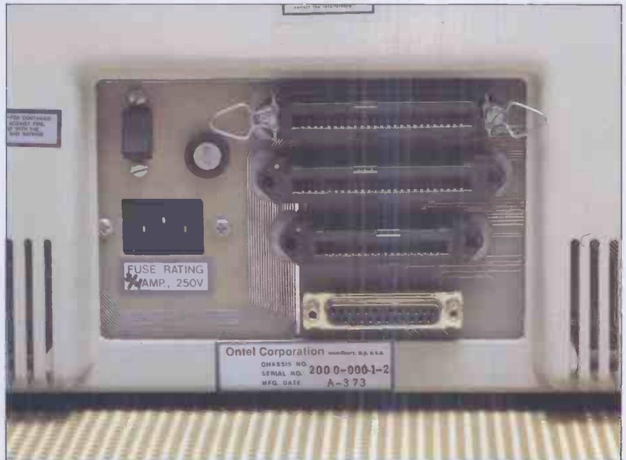
Top to bottom: floppy disk connector, hard disk controller, Centronics and RS232 ports.
