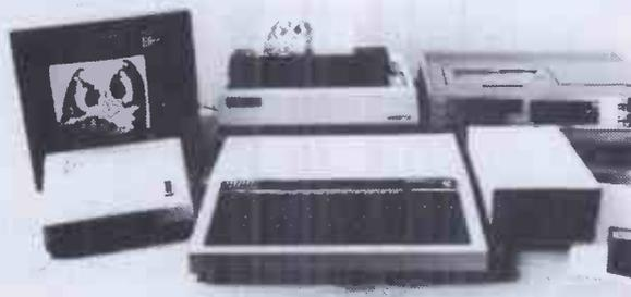
256 x 256 pixel resolution with 255 grey levels per pixel comes complete with software and documentation. Can be used for video tape digitising Satellite picture analysis etc. Available for BBC, Apple, Commodore, Research Machine, Sirius etc.
