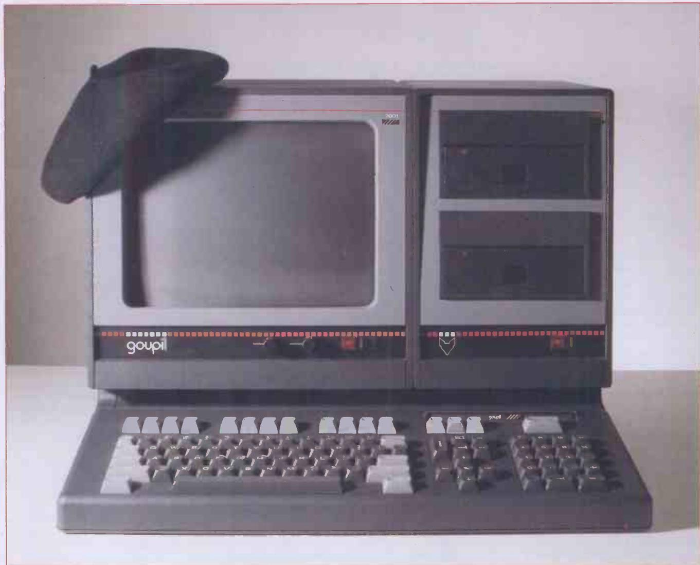
The Goupil-3 is a modular computer system designed to cater for both professional and personal needs. Its building block design allows the user to build up a computer system from the simple screen, console and keyboard configuration to a fully expanded system supporting three processors, a choice of six operating systems and offering multi-user and multitasking facilities.
