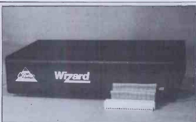
The Colour Genie micro now has a diskette interface (shown here), price £90, which includes a parallel printer interface.
