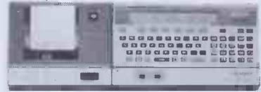
3.5K RAM (2.6K user) expandable; 16K ROM. BASIC Mini-Graphic display. Up to 36 program storage; Full math, science, clock and beep functions; Auto power off, with memory protection.
