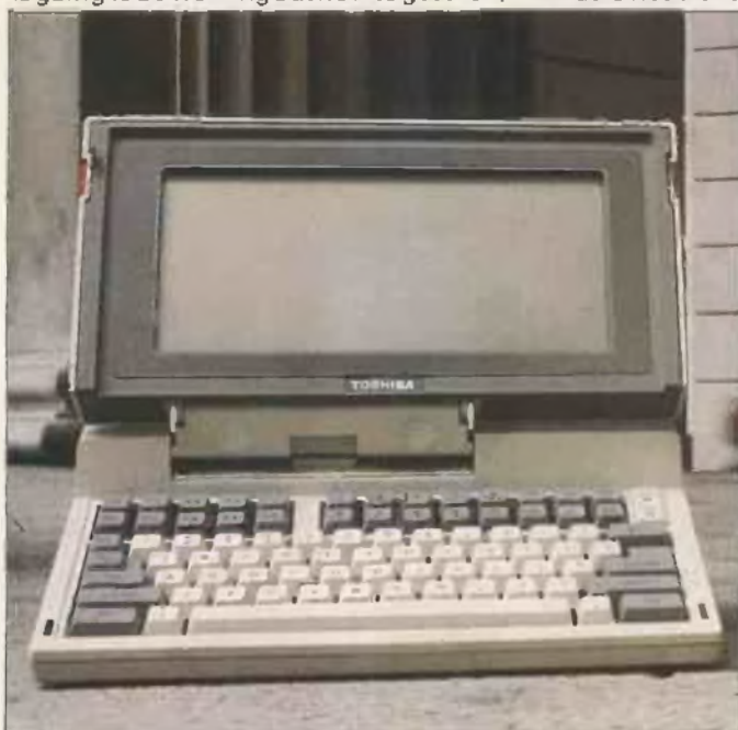
A powerful hinge allows the machine to be easily tilted
