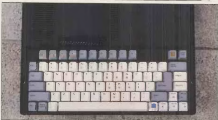
The Kaypro's ten function keys form a single row above the keyboard
