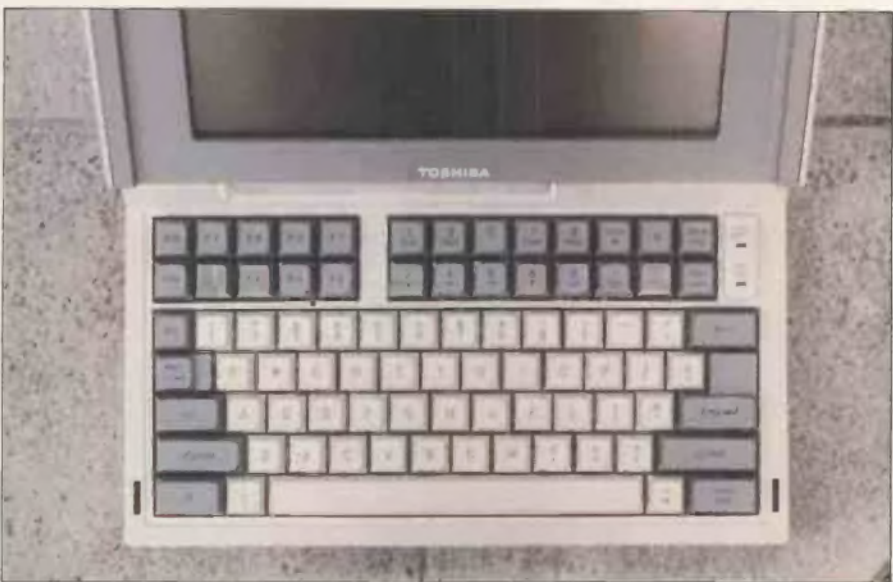
Unfortunately the ALT and CAPS lock keys are still level with the space bar
