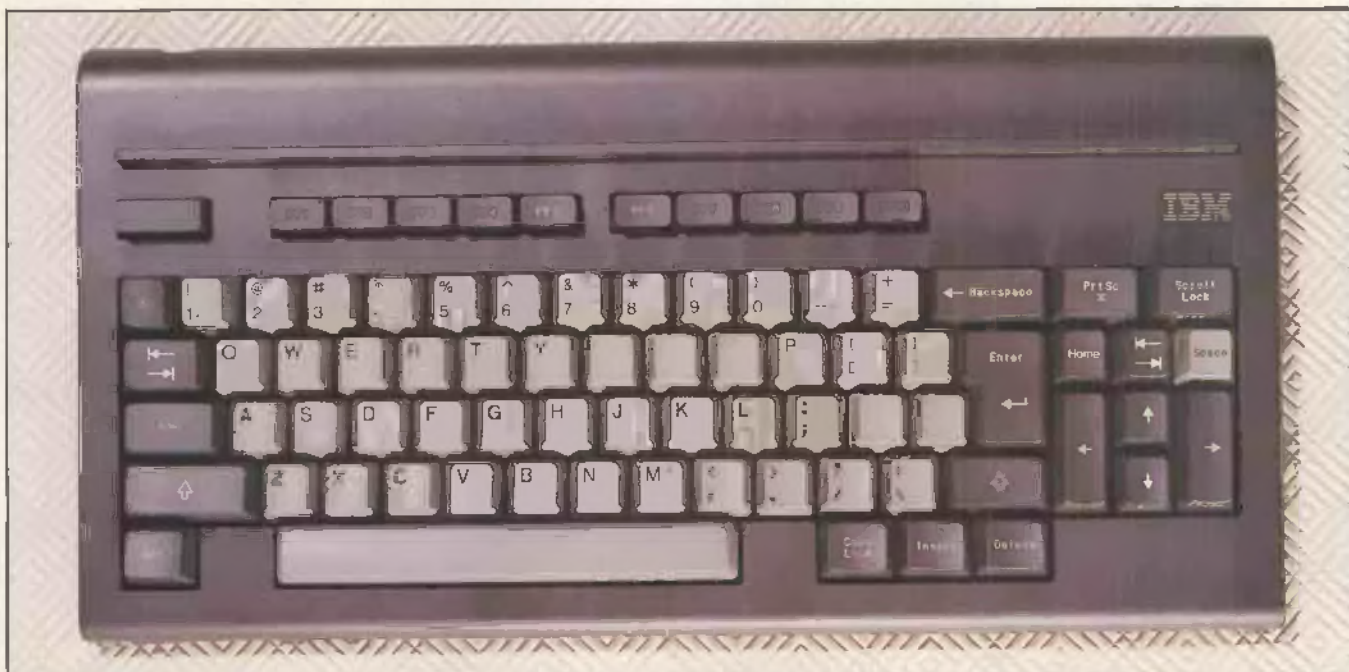
The JX's keyboard is of a light construction but has a positive feel, and provides infra-red or cabled operation.
