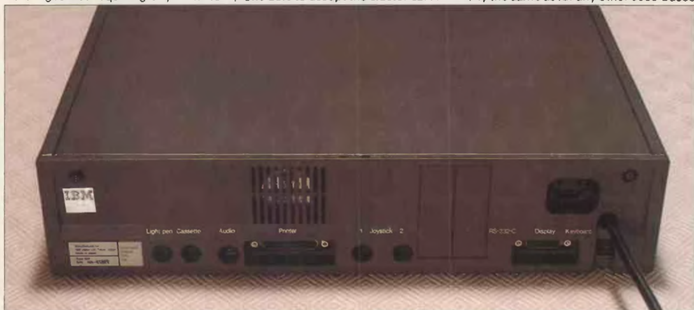
Optional device ports are included for a cassette, light-pen memory expansion and asynchronous communications
