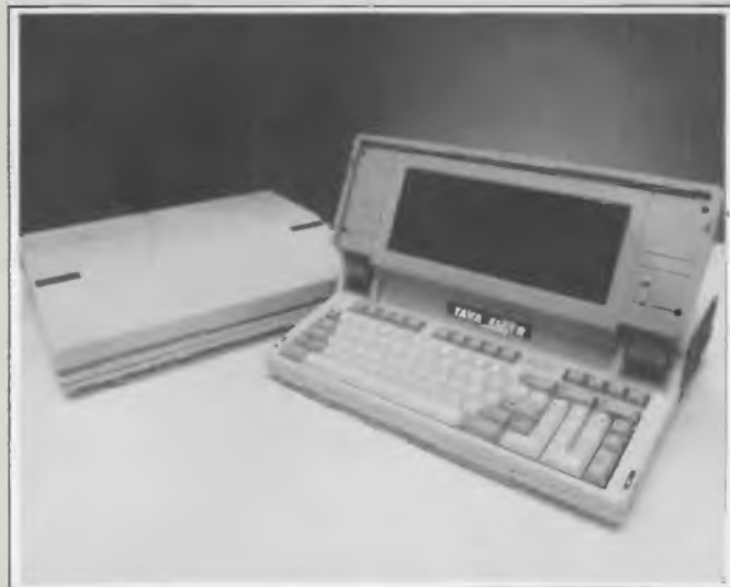
The New Tava Flyer Winchester disk based portable computer. The Tava Flyer features 20 MBs of integral Winchester storage, back lit screen and facilities for coaxial connection to IBM mainframes.
