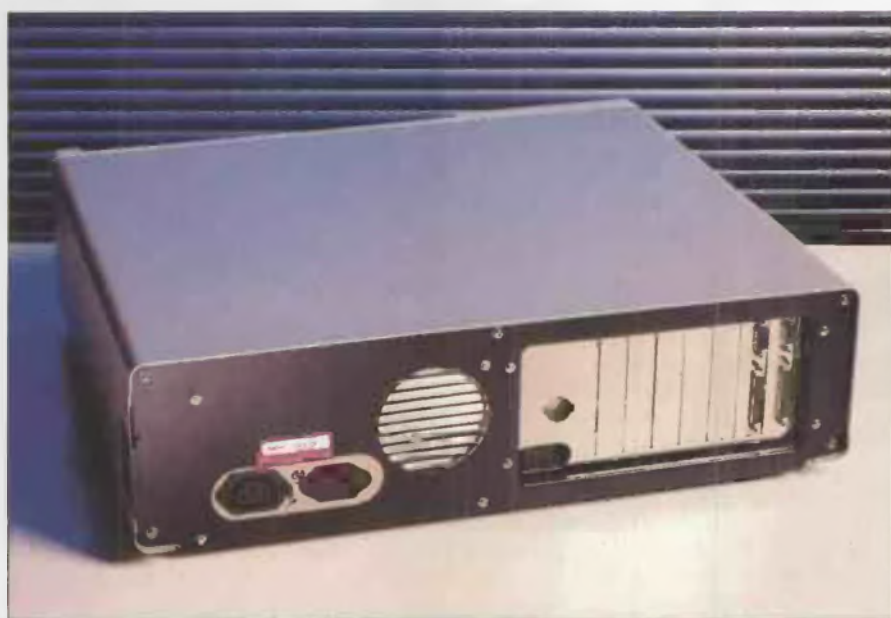
Expansion slots include a combined memory/input-output board
